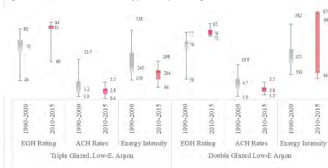
Figure 4. Percentage box plot shows minimum, 25% percentile, median, 75% percentile and maximum values for performance parameters between 1990 to 2015 comparing triple glazed to double glazed windows. Values for minimum, median and maximum are labelled on the graph.
