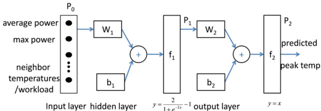
**Figure 4.5 Neural network predictor architecture**
