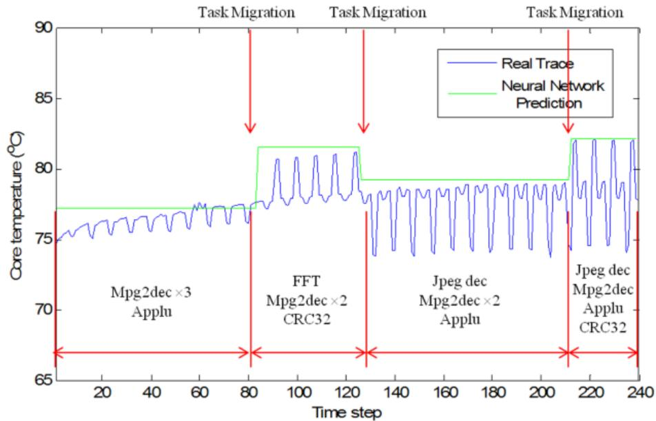
**Figure 4.7 The temperature prediction of neural network model**
