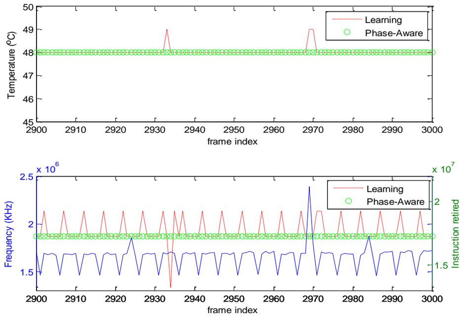
**Figure 3.5 Temperature and frequency comparison between Learning and Phase-Aware**
