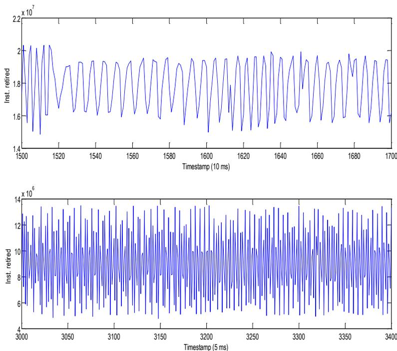
**Figure 3.1 Variation of retired instructions for every 10 and 5 ms for MPEG4 decoder**
