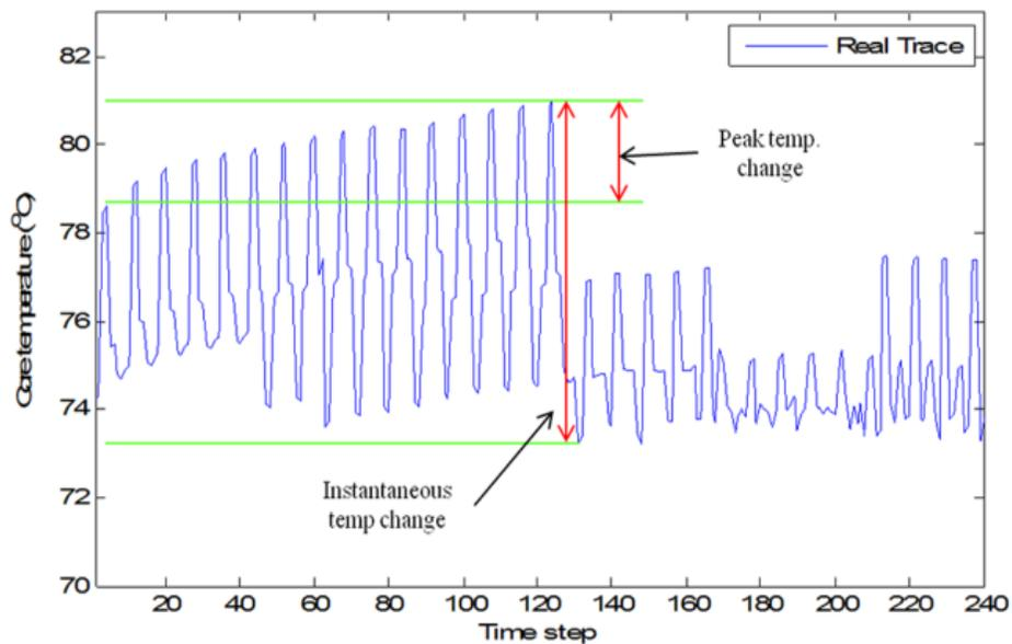
**Figure 4.3** Example of instantaneous and peak temperature change
