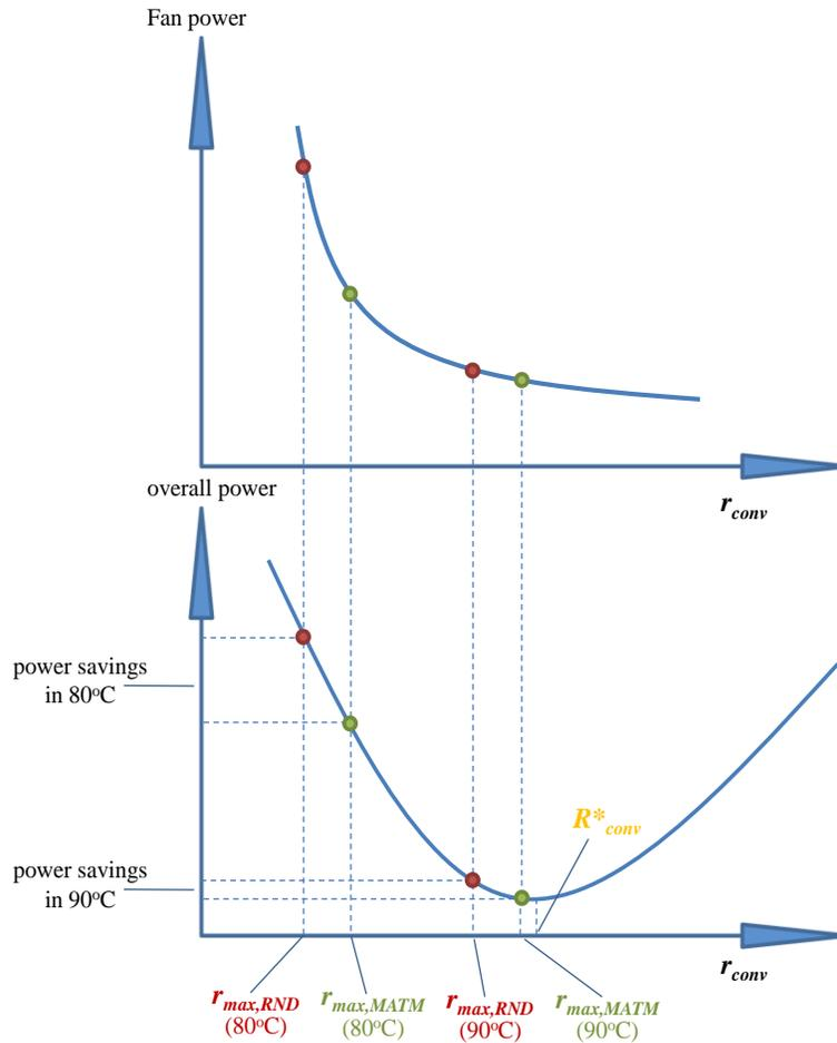
**Figure 5.9 Power consumption against convective thermal resistance curve**
