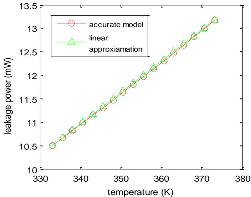
**Figure 5.3 Linear approximation of leakage power model**
