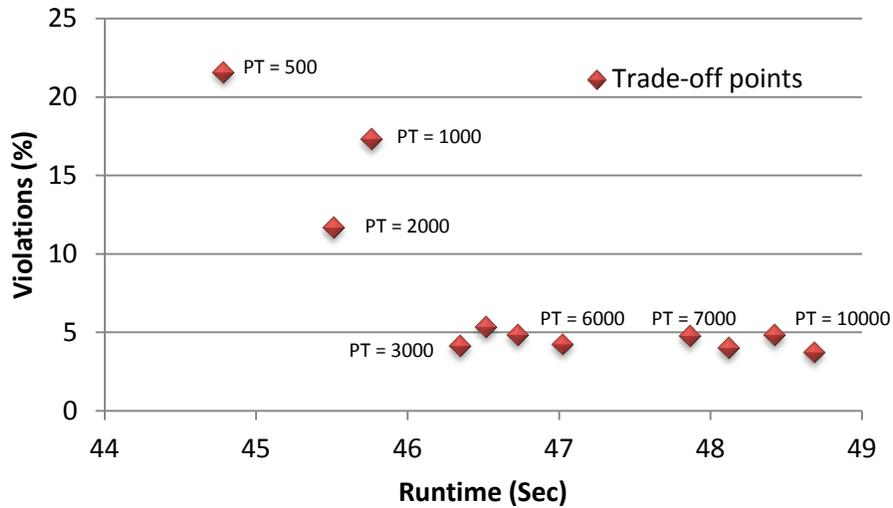
**Figure 3.7 Trade-off between run time and thermal violation**
