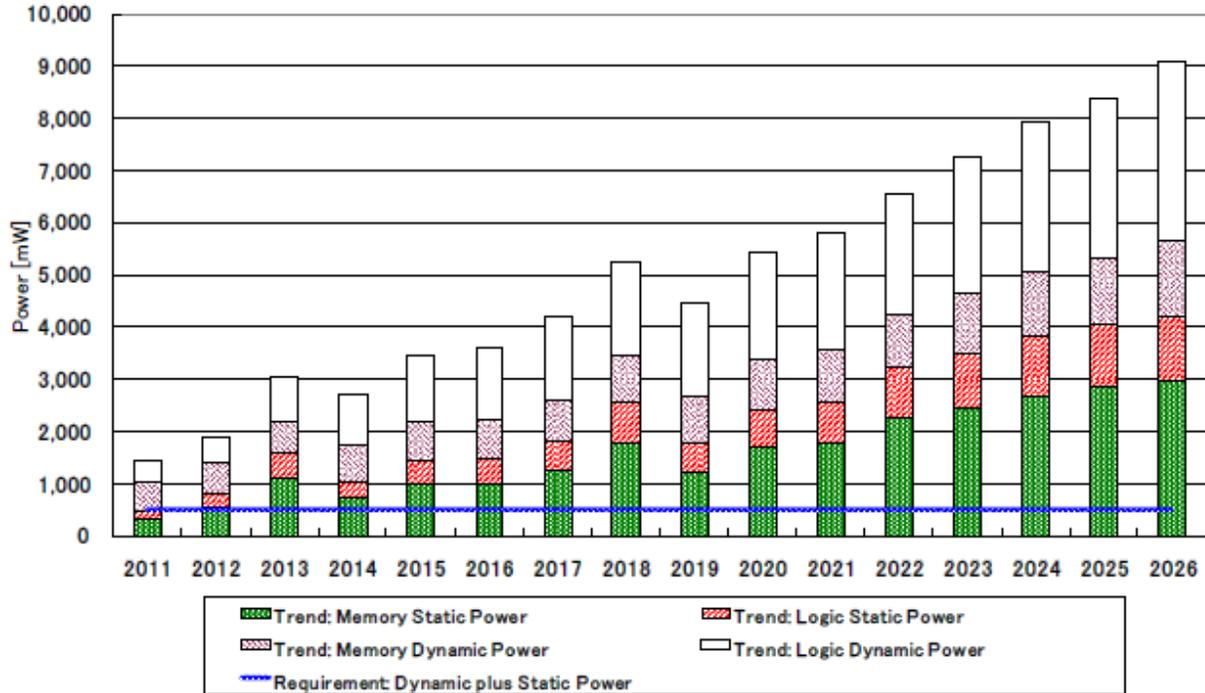
**Figure 1.1 System-on-Chip (SOC) Consumer Portable Power Consumption Trends [4]**
