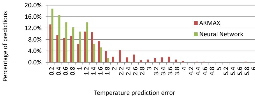
**Figure 4.10 Comparison of peak temperature prediction error**
