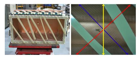
Fig. 2. Left: The ArgoNeuT TPC. Right: Wire orientations of ArgoNeuT TPC (Collection=-60°, Induction=+60°)
