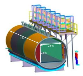
Fig. 3. Schematic diagram of MicroBooNE experiment.
