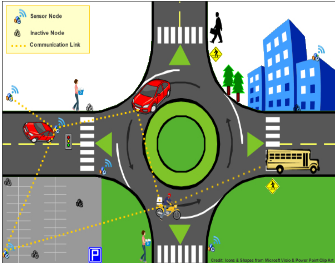
Figure 4.3. Vehicular Ad-hoc NETWORK (VANET)
