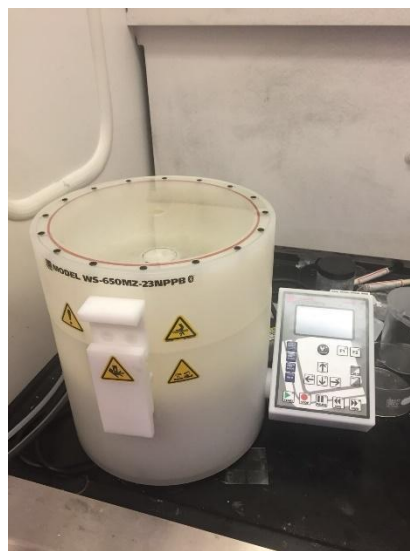
Figure 21 The PEM film is coated onto the stretched polymer in the spin coater.
