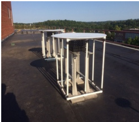
Figure 2.2: The two disks deployed in the field. Each disk is ~ 2.5 m away from the penthouse and the railing. The disks are supported underneath by a frame of PVC pipe secured to concrete pavers.
