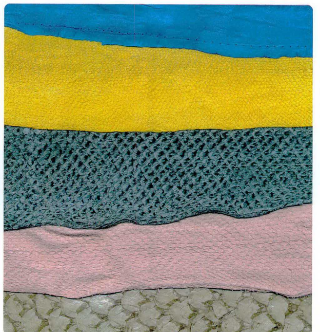
Fig. 10. Commercially tanned skins. From the top: eel, trout suede, salmon glazed, salmon suede, carp glazed.
