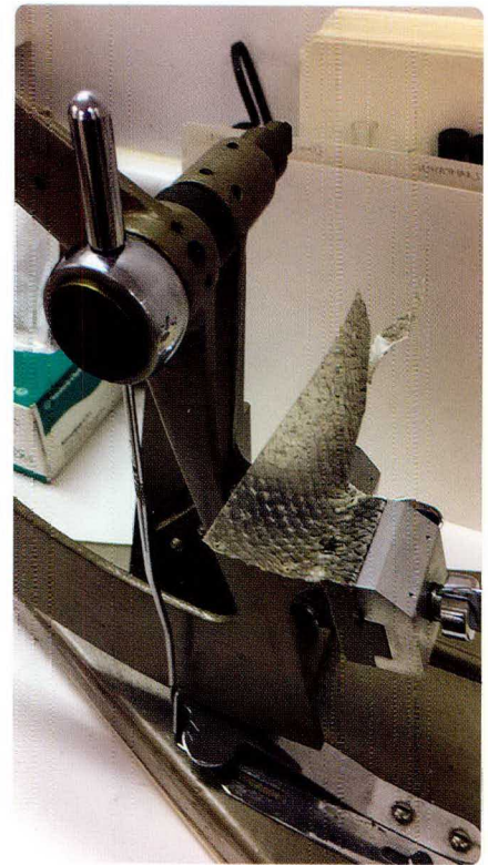
Fig. 3. Elmendorf tear tester showing a 'failed test' on the salmon: the fish skin was too strong. Photo: Timothy Barrett.
