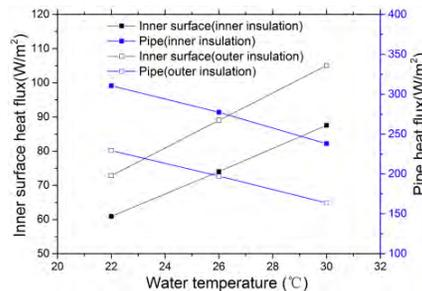
Figure 5. Influences of insulating layer with different locations
