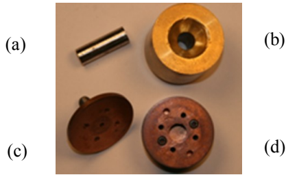
Fig. 2: Actual picture of the different parts of fabricated test setup. (a) plunger. (b) Plunger support. (c) Coaxial lines of regions I to III. (d) Hollow circular waveguide, region IV. Part (a) goes into (b) on top of (d) to pack the powder inside (d), then removed. Measurements are realized when part (c) is ended with part (d) filled with powder.
