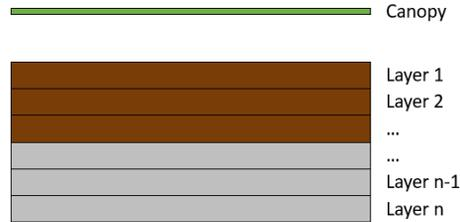
Figure 1. Discretization of the different layers of the VR (Brown and grey layers correspond to the substrate and concrete slab structure, respectively)
