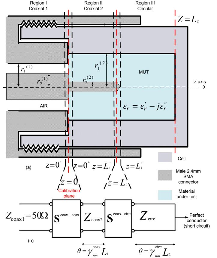
Fig. 1. (a) The schematic of test setup. (b) Generalized scattering matrices building blocks. Dimensions of design parameters are:  $r_1^{(1)} = 1.2$  mm,  $r_2^{(1)} = 0.52$  mm,  $r_1^{(2)} = 1.26$  mm,  $r_2^{(2)} = 0.254$  mm,  $L_1 = 1.1$  mm,  $L_2 = 5.3$  mm.
