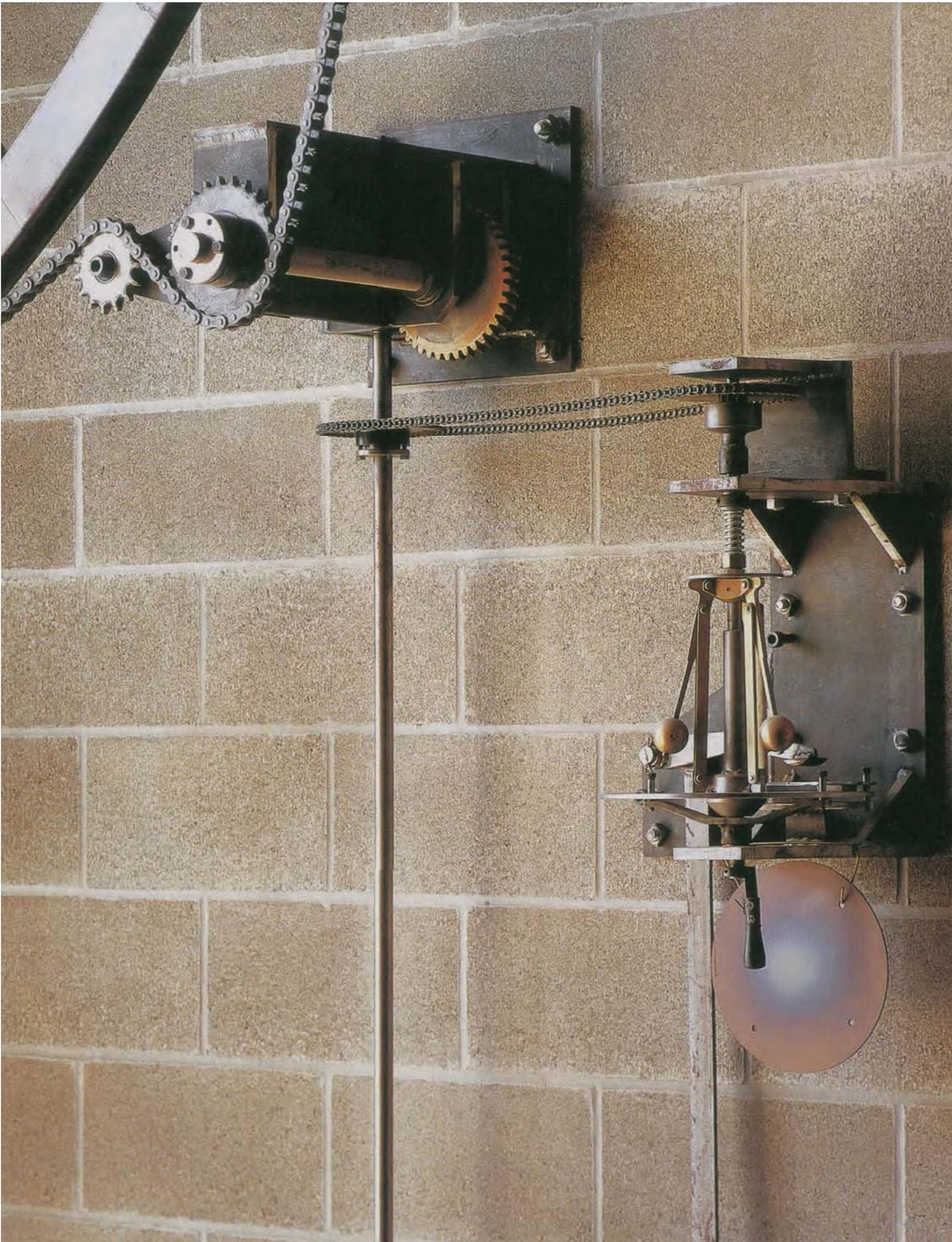
Figure 118: Detail of the gear mechanism, flyball governor, and the steel plate ringer that hangs below it.
