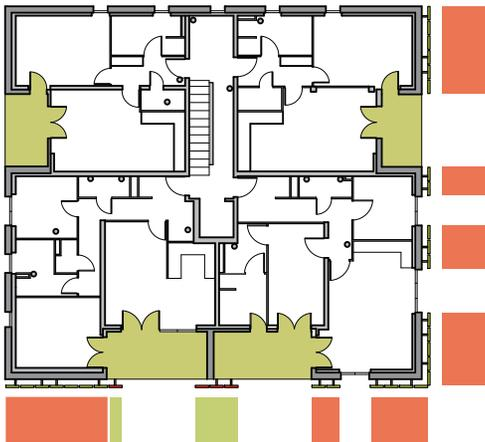
Figure 28 . Second floor plan corresponds to exposed and wall panels and interior porches are painted green.
