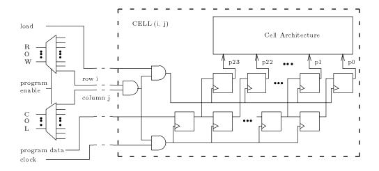
Figure 2: FPGA Programming Logic and Cell Program Memory
