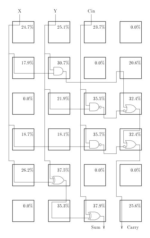
Figure 4: Mapped Full Adder. Percentages are individual cell fault coverages achieved by applying an exhaustive set of mission test vectors.
