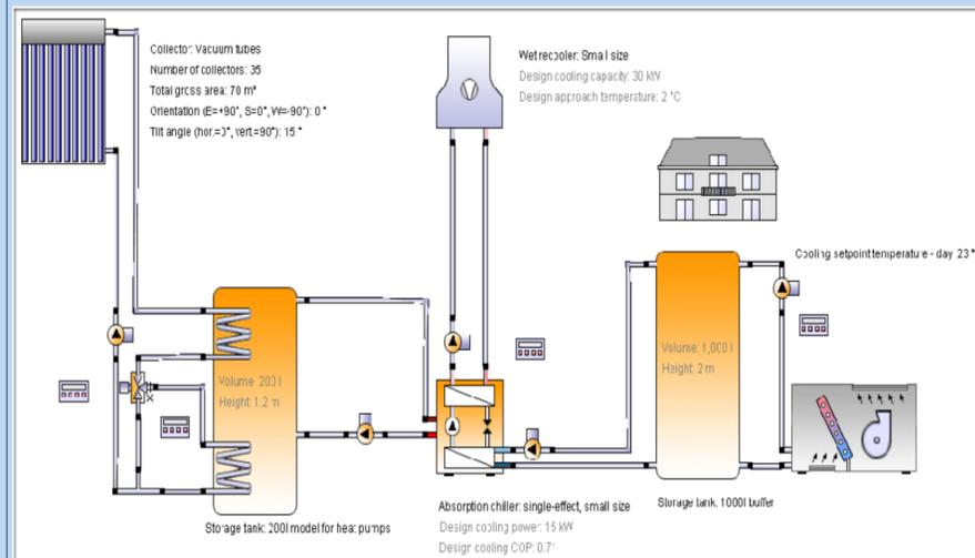
Figure 3: Solar thermal cooling system simulation model (Fathhee & Jiang, 2021)
