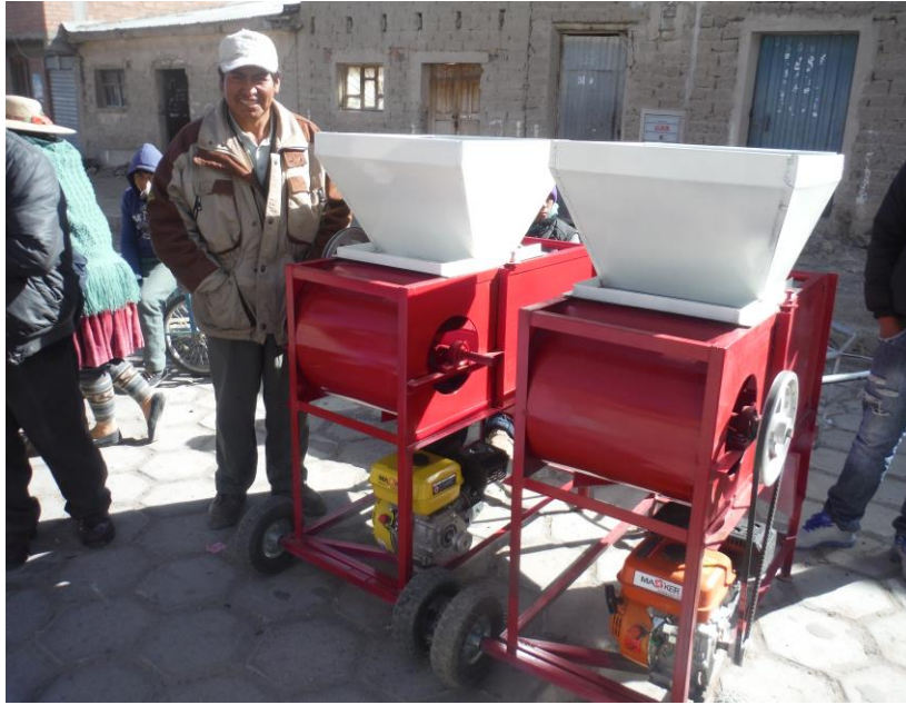
Photo 2.1: An example of a venteadora (a machine that sorts quinoa) with a motor. Photo taken by author in a market in the town of Challapta of the Province of Oruro.
