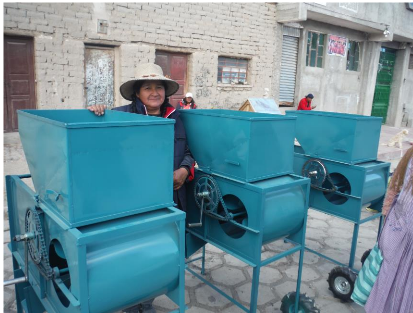
Photo 2.2: Venteadoras without motors, powered by hand cranks. Photo taken by author in the same market, just across the street from the photo above.
