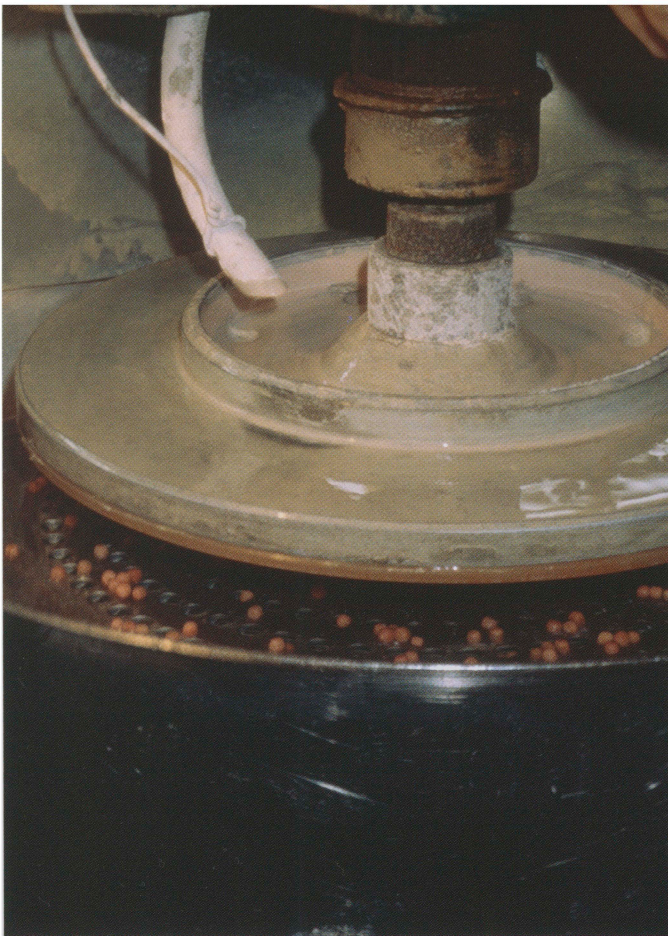
Plate IIA. Coral: Pallini in the rociatrice machine. The holes in the lower disc secure the coral pieces while the grindstone reduces them to the proper size (photo by author).
