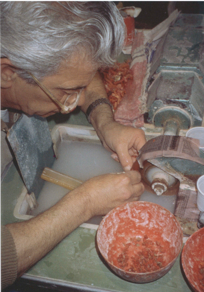
Plate IC. Coral: Branch sections are formed into bead blanks by cutting progressively smaller pieces on an electric saw. The cutter's skill and expertise determine the final disposition and preparation of the piece of coral (photo by author).
