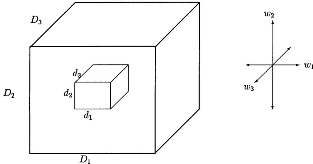
Figure 2: Iteration Space  $D_1D_2D_3$ , Block  $d_1d_2d_3$ , and Communication Weights  $w_1$ ,  $w_2$ ,  $w_3$
