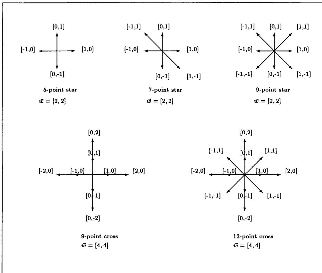
Figure 3: Discretization Stencils and Communication Weight Vectors
