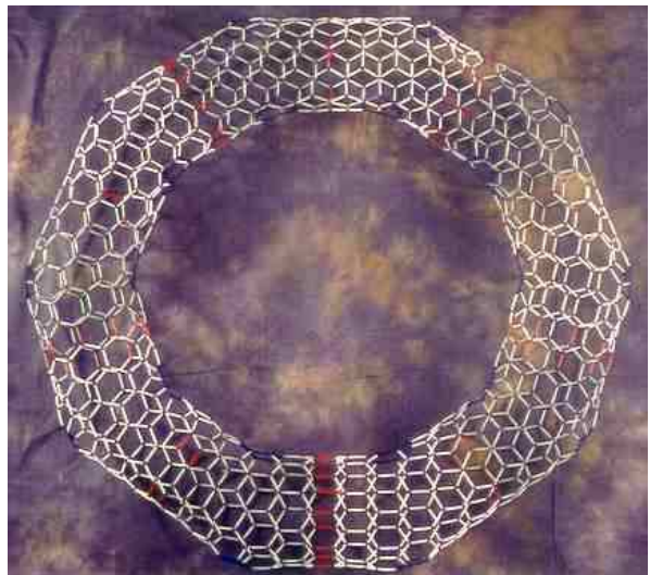
FIG. 5: (Color online) Five-fold polygonal torus obtained by joining (5, 5) and (9, 0) tubular segments via ten pairs of 5–7 rings. This structure was originally proposed by the authors of Ref. 27 as a possible low-strain configuration for carbon nanotori. [Courtesy of A. A. Lucas and A. Fonseca, Facultés Universitaires Notre-Dame de la Paix, Namur, Belgium].
