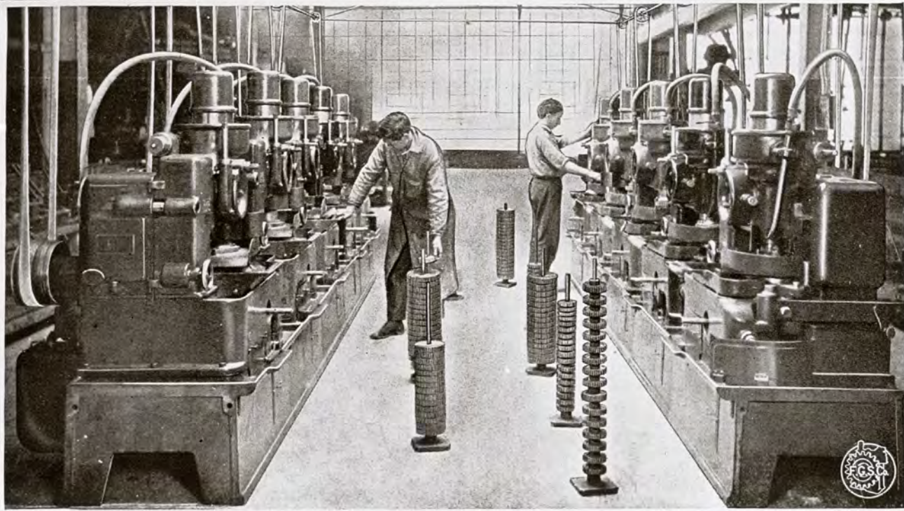
Illustrating Battery Installation of New High-speed Gear Shaper One 6-H.P. Motor furnishes Ample Power for Ten Machines
