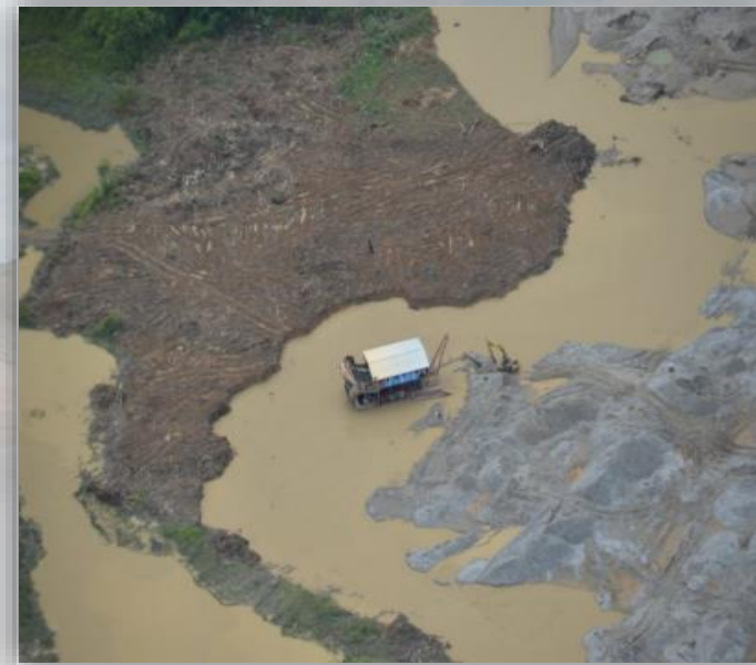
Figure 2. Gold mining in the Atrato river - Choco by using dredges and adding mercury. Source: [1].
