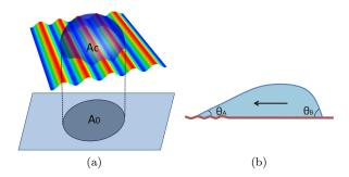
FIG. 1: (a) A liquid droplet sitting on a rough substrate has more contact area with the substrate  $(A_c > A_0)$  than the same droplet on an otherwise identical flat substrate. (b) A liquid droplet partially wetting a hydrophilic substrate with inhomogeneous roughness has a smaller contact angle at the rougher end  $(\theta_A)$  than at the smoother end  $(\theta_B)$ .
