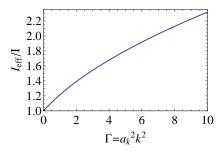
FIG. 3: The ratio of the effective imbibition parameter to the physical imbibition parameter versus  $\Gamma = a_k^2 k^2$  for a liquid droplet partially wetting a sinusoidally modulated substrate.
