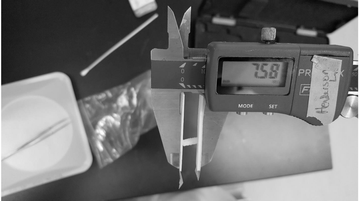
Figure 2-3. Preliminary foam compression method. Involved manually compressing and measuring each foam simultaneously which turned out to be time consuming and inaccurate. Samples would have a tendency to become dislodged during compression because the applied force was non-uniform. Additionally, samples would prematurely recover their uncompressed shape because there was no step for precisely fixing the temporary compressed shape.
