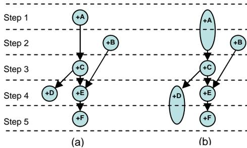
Figure 5: Two possible schedules for the data-flow graph<sup>\*</sup> shown in Figure 4(a).
