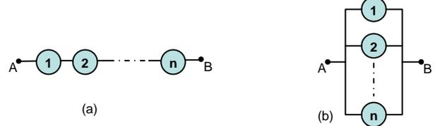
**Figure 3: Serial (a) and parallel (b) reliability models.**
