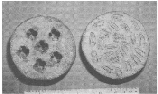
Figure 3. The mold on the left is for making the base of a zagba type. The one on the right is used to make decorative components (Kirk Stanfield collection; photo: Robert K. Liu).
