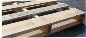
224 GMA wooden pallets [wall modules]
