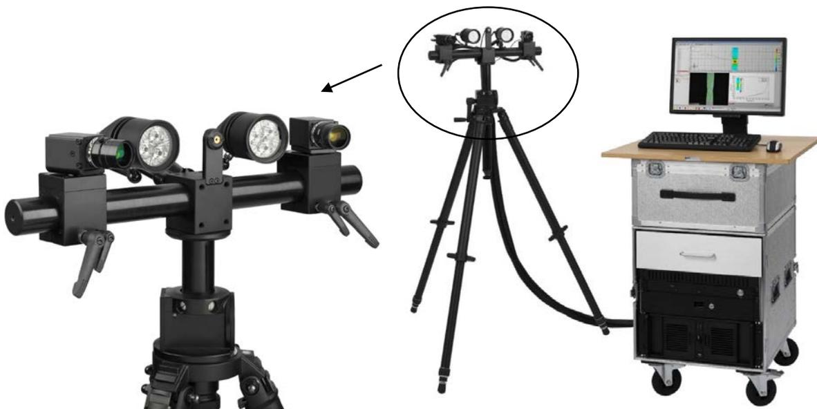
Figure 4.1. ARAMIS Camera Bar and Computer Setup
