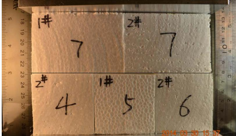
Figure 5.5. Five EPS Blocks with Mixed 1&2pcf EPS Stacked in 2 Layers without Continuous Vertical Joints
