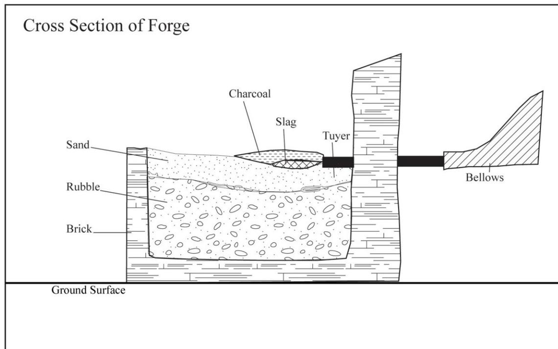
**Figure 3:3 Idealized cross section of a forge illustrating the construction layers within the forge's hearth bed and the location of the *tuyère* and bellows. Redrawn after Light 1987.**
