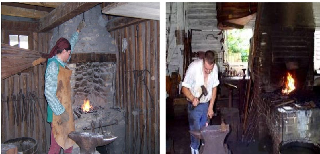
**Figure 3:4 Examples of bellows positions. Reenactor from Fort Michilimackinac working with a side mounted bellows system (left) and a reenactor from Colonial Williamsburg working with a rear mounted bellows system (right). Photos taken by the author.**
