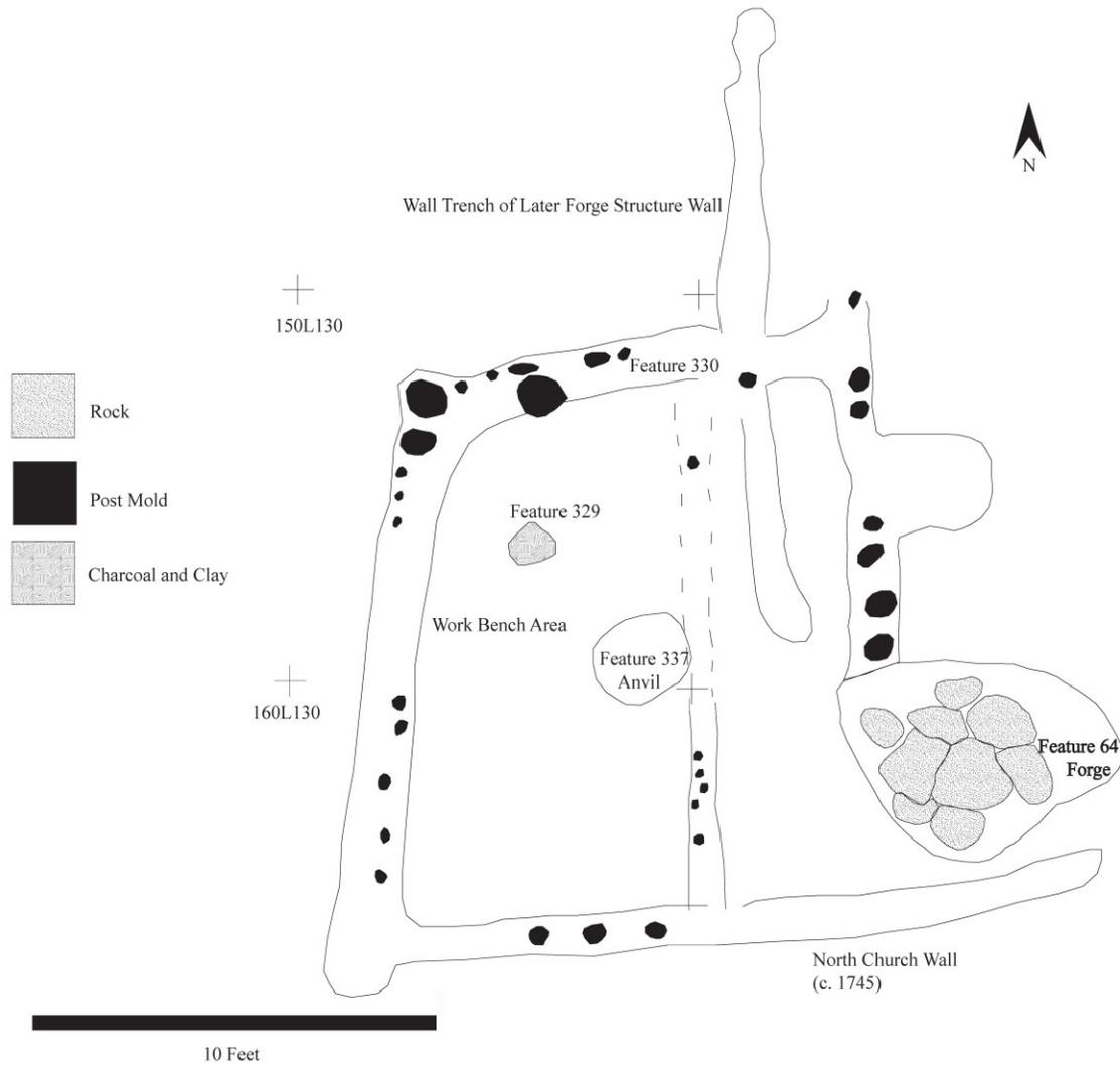
**Figure 4:4 Activity areas related to blacksmithing and gunsmithing in locus A were identified following the application of the blacksmith workshop model. Reinterpreted from a compilation of Stone (1966), Brown (1967), and plan maps.**
