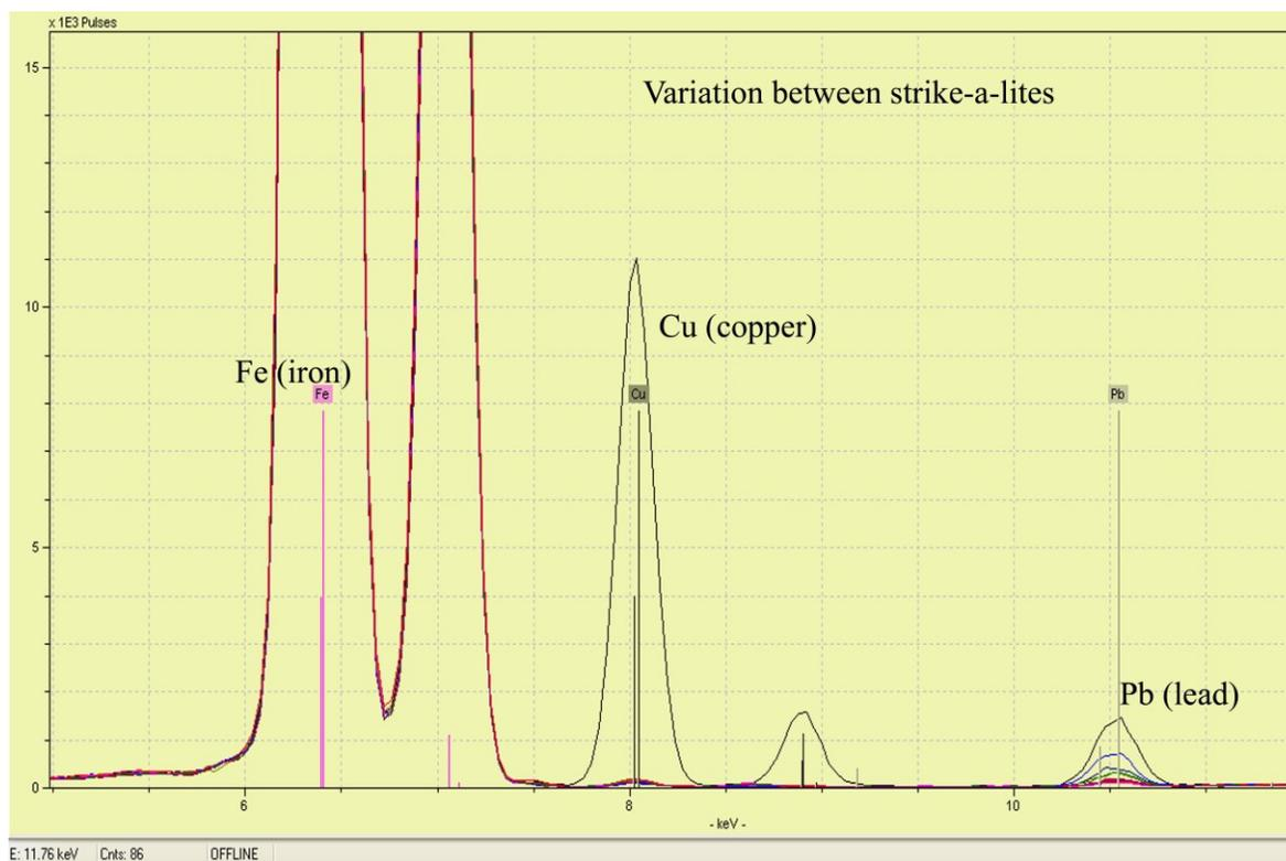
**Figure 5:15 Raw data pXRF showing variation between strike-a-lites from Fort Michilimackinac.**
