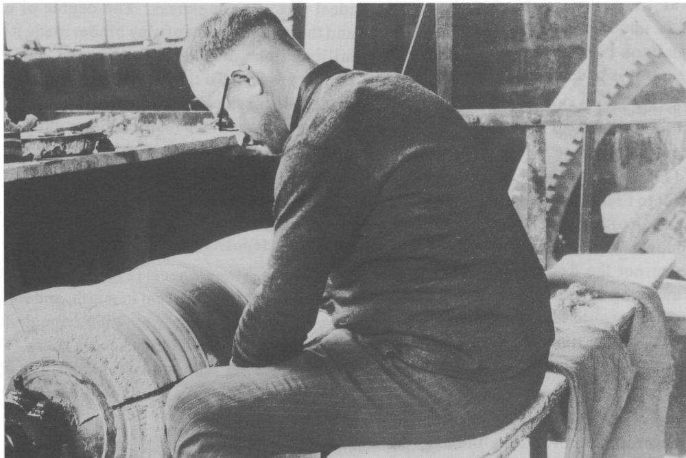
Figure 8. Polishing gems on a beechwood cylinder. Part of the elaborate gear-and-belt system which transferred power from the water wheel to the equipment is visible in the background.
