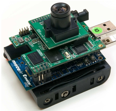
Figure 1.8: CITRIC embedded smart camera Mote
