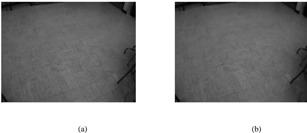
Figure 6.9: QVGA images captured by (a) using the API software library down-sampling subroutines and (b) performing hardware-level down-sampling on the micro-controller of the OV9655.
