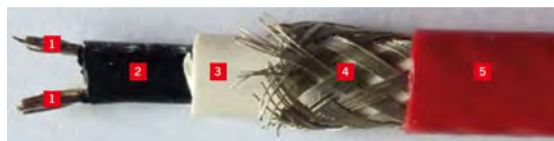
Figure 4 A self-regulating heating cable with possibility of adapting heating power to ambient temperature. 1-power supply cables, 2-conductive polymer, 3-insulation cover, 4-screen, 5-outer cover.
