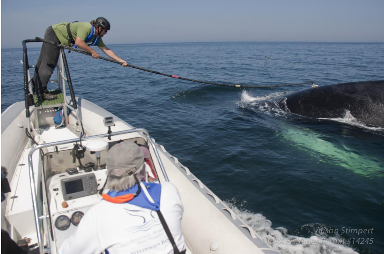
Figure 1: A handheld 7 m carbon fiber pole is used to place the DTAG onto a humpback whale's back. (Photo credit: A. Stimpert, NOAA Fisheries Permit #14245)
