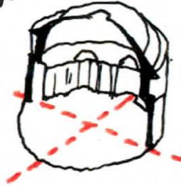
b. stone dome on circular plan, the purest form of geometry
