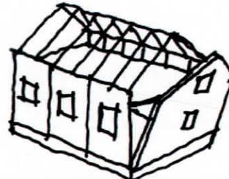
g. prefabricated panel construction becomes a quick and cheap solution to housing
