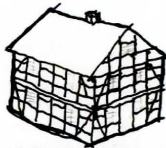
f. the introduction of timber allows the isolation of windows, while building corners were supported by corner struts and walls contained straw, mud, or clay
