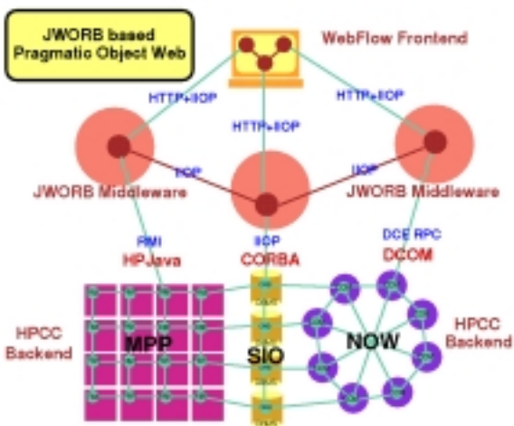
Figure 1: Support for multiple protocols and heterogeneous backend services within the JWORB based Pragmatic Object Web.
