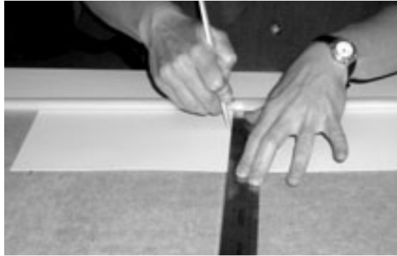
Creasing the folder stock on the jig.
