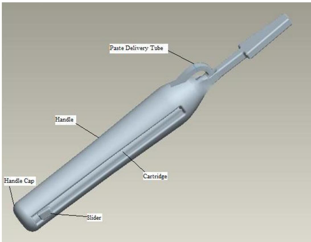
Figure 13: 3-D model of the toothbrush
