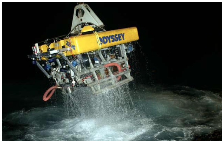
ROV ZEUS used to excavate SS REPUBLIC
