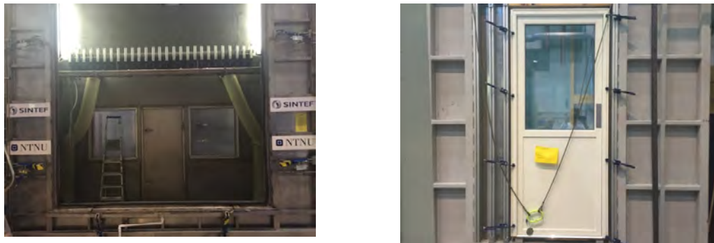
Figure 3. Test equipment for testing according to EN 1027. (left) nozzle system. (right) an example of a door mounted in the apparatus.
