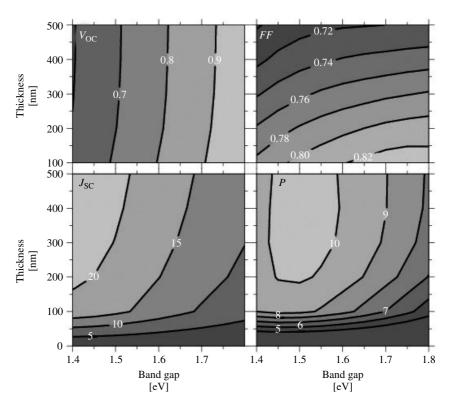
**Figure 12.20** Model calculations of the short-circuit current  $J_{SC}$  (mA/cm<sup>2</sup>), open-circuit Voltage  $V_{OC}$ , (V), fill factor FF, and power P under AM1.5 illumination for a-Si:H-based pin solar cells with varying intrinsic layer band gaps and thicknesses. No back reflector or texturing effects are included
