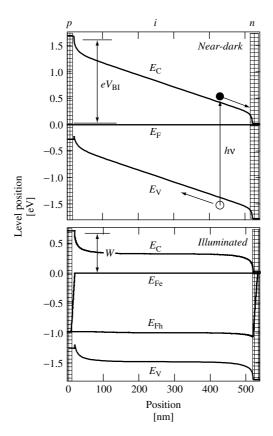
**Figure 12.14** Bandedge and Fermi-level profiles in a *pin* solar cell under open-circuit conditions. The open-circuit voltage is precisely the value of  $E_{\rm Fh}$  at the left interface (x=0). The built-in potential  $V_{\rm BI}$  is illustrated. Note that the *p*-layer has a slightly (0.2 eV) larger band gap than the i-layer; the calculation assumes symmetrical offsets of the valence and conduction bands at the p/i interface
