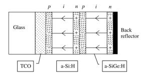
**Figure 12.4** A multijunction solar cell consisting of two *pin* solar cells deposited in series. Double-junction (or "tandem," as shown) and triple-junction designs can be significantly more efficient than single-junction designs. Substrate texturing, which is important in real devices, is not indicated; see Section 12.4.5
