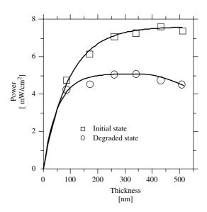
**Figure 12.21** Power output (standard solar illumination) for a series of *nip* solar cells with varying intrinsic layer thickness [14]. The degraded state was obtained by 25 000 h of light soaking. The curves are guides only
