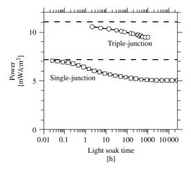
**Figure 12.5** The conversion efficiency in a-Si:H-based solar cells declines noticeably upon the first exposure to sunlight. The figure illustrates this decline under a solar simulator ( $100 \text{ mW/cm}^2$ ) for a single-junction cell (260 -nm i-layer thickness) and for a triple-junction module made at United Solar Systems Corp. [14, 15]; the dashed lines indicate the initial power measured for each device
