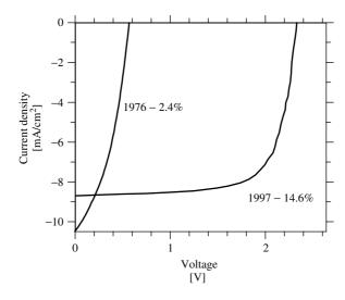
**Figure 12.1** Current density versus voltage under solar illumination for a very early single-junction amorphous silicon solar cell (Carlson and Wronski [5]) and from a recent "triple-junction" cell (Yang, Banerjee, and Guha [8]). The stabilized efficiency of the triple-junction cell is 13.0%; the active area is 0.25 cm<sup>2</sup>
