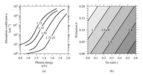
**Figure 12.10** (a) Absorption coefficient spectra for a-SiGe alloys; the optical band gaps and corresponding Ge fractions x are 1.25 to 0.58, 1.34 to 0.48, 1.50 to 0.30, 1.72 to 0.0 [52]. (b) Typical optical band gaps for a-Si<sub>1-x</sub>Ge<sub>x</sub>:H alloys for varying Ge-ratio x and atomic fraction h of hydrogen
