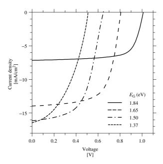
**Figure 12.23** Performance of a-Si and a-SiGe nip solar cells with different Ge concentrations in the i-layer; the i-layer band gaps are indicated in the legend. The fill factors for these cells are 0.70, 0.62, 0.55, and 0.43 for the cells with i-layer band gaps of 1.84, 1.65, 1.50, and 1.37 eV, respectively [149]
