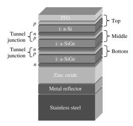
**Figure 12.25** Structure of triple-junction *nip* substrate-type solar cells
