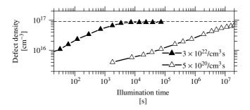
**Figure 12.8** Plot of the defect (dangling bond) density during extended illumination of an a-Si:H film as measured by Park, Liu, and Wagner [34]. Data are given for high- and low-intensity illumination; the legend indicates the photocarrier generation rate of each intensity
