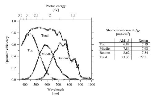
**Figure 12.26** Quantum efficiency curves of component cells of a typical triple-junction solar cell. The table indicates the short-circuit current densities  $J_{SC}$  for the component cells measured for AM1.5 illumination and with a xenon illuminator [158]
