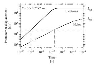
**Figure 12.15** Displacements (or drift lengths) of electron and hole photocarriers in a-Si:H as a function of time following generation at room temperature [41]. Note that displacements are proportional to electric field. The saturation in the displacement for longer times (at  $L_{e,t}$  and  $L_{h,t}$ ) is due to deep trapping of electrons and holes by defects. Dotted lines illustrate the time required to drift 250 nm
