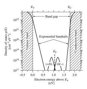
**Figure 12.9** Density of electronic states g(E) in hydrogenated amorphous silicon. The shaded areas indicate delocalized states in the bands; these bands themselves have tails of localized states with an exponential distribution. Midway between the bands are levels belonging to gross defects such as dangling Si bonds indicated by the two peaked bands around  $E_F$
