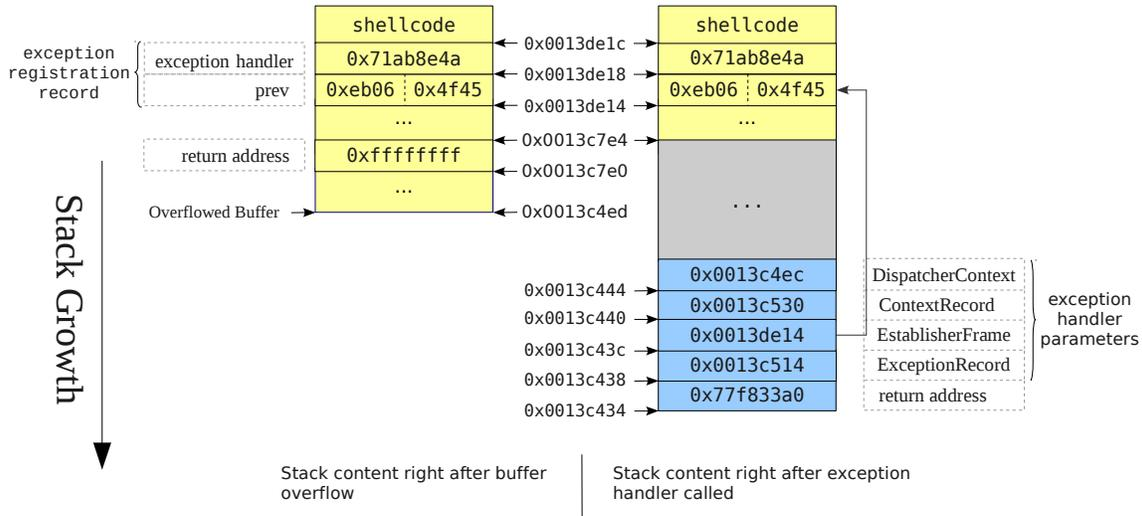
Figure 1. Stack layout in an SEH exploit.
