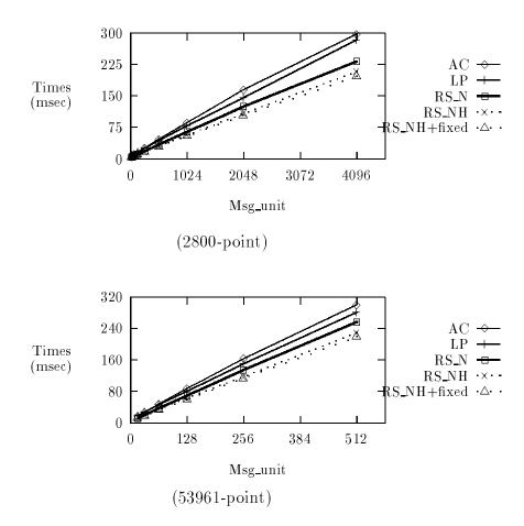
Figure 16: Communication cost for airfoil mesh simulation on a 32-node CM-5.
