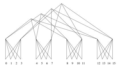
Figure 3: CM-5 data network with 16 nodes.
