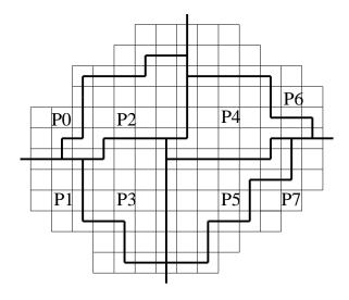
Figure 2: The partitioning of irregular mesh.
