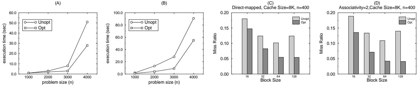
Figure 8: (A) Execution times for *simple-transpose* on RS/6000. (B) Execution times for *simple-transpose* on SPARCstation 5. (C) Miss ratios for the LU decomposition. (D) Miss ratios for the LU decomposition.
