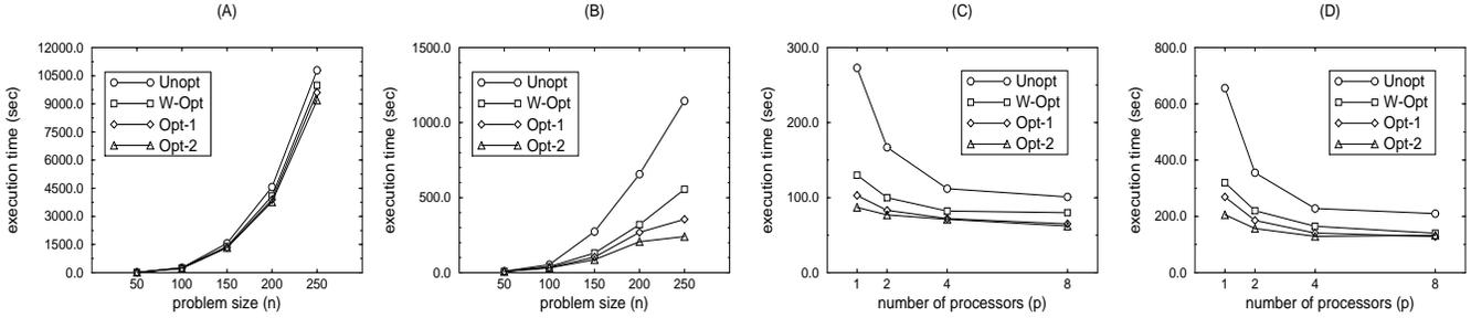
Figure 6: Execution times (A) on SPARCstation 5. (B) on a single node of SGI. (C) on multiple nodes of SGI with  $150 \times 150$  double arrays. (D) on multiple nodes of SGI with  $200 \times 200$  double arrays.
