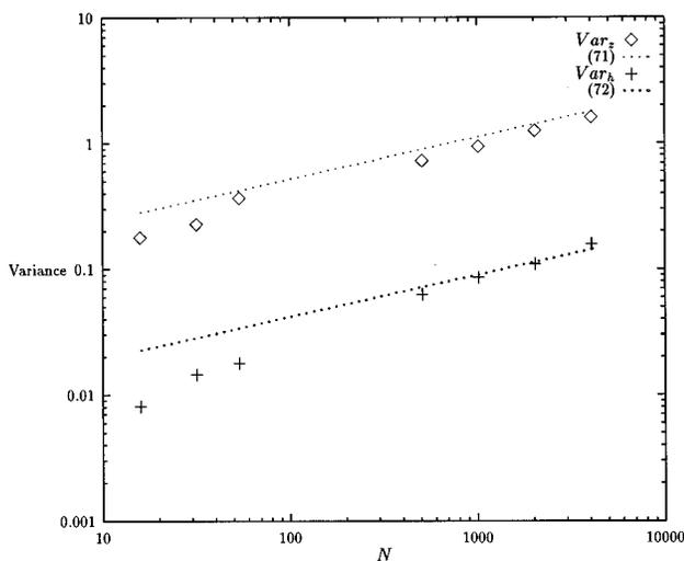
FIG. 6. The divergence of velocity variance with the system size  $N$  in random sedimenting suspensions with  $\phi=0.05$ . The top line corresponds to the theoretical prediction for the velocity variance in the direction of gravity while the bottom line corresponds to the velocity variance in the plane normal to gravity.
