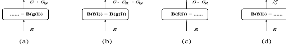
Figure 10: Handling communication during backward analysis in a node using different approaches: (a), (b), and (c) by the approach given in Figure 7; (a), (b), and (d) by the approach given in Figure 11.
