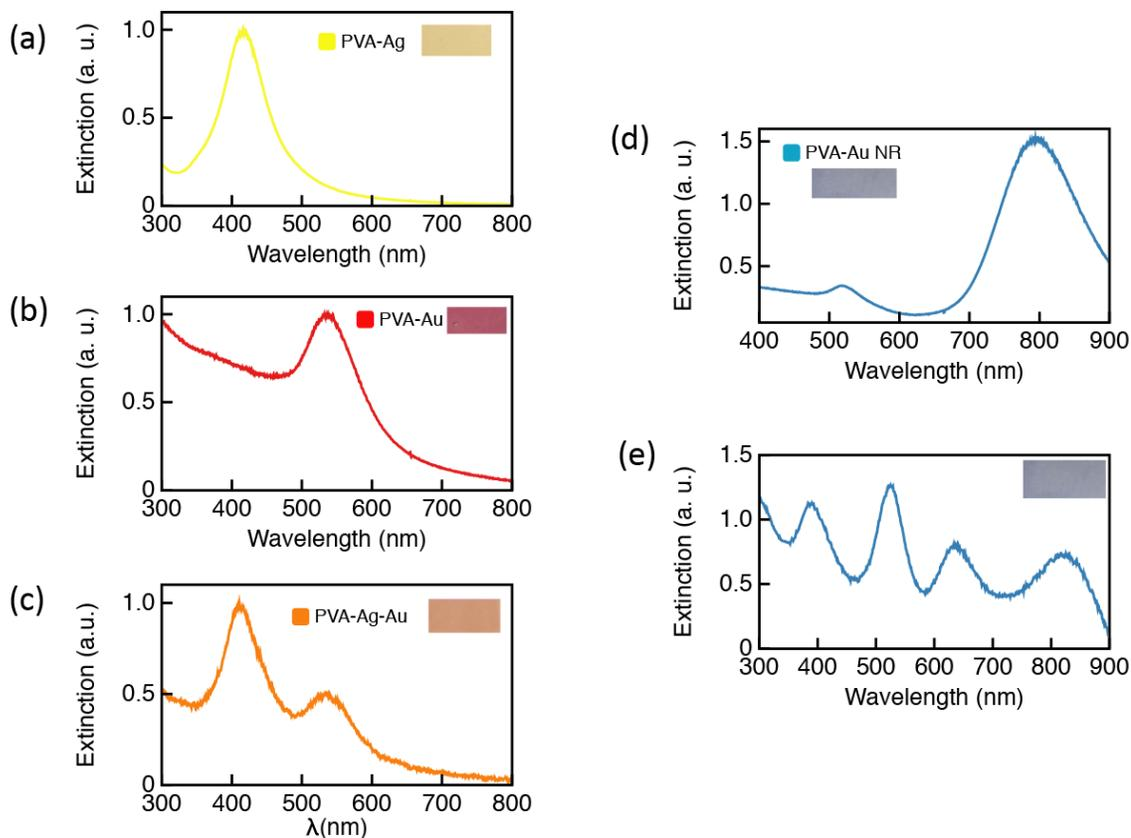
**Figure 5–8: Extinction spectra of flexible plasmonic nanofilms containing different types of nanoparticles. (a) Ag nanospheres; (b) Au nanospheres; (c) Au and Ag nanospheres; (d) Au nanorods; (e) a mixture of four types of nanoparticles.**
