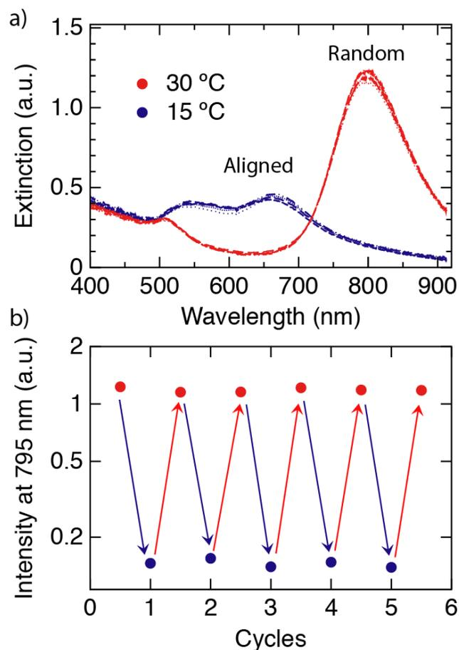
**Figure 4–3: a) The extinction spectra of an Au nanorod suspension during six cycles of repeated heating (at 30 °C) and cooling (at 15 °C). b) The repeated switching of extinction intensities at 795 nm for six cycles.**
