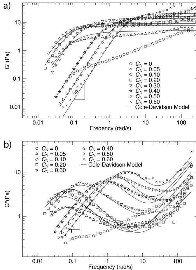
**Figure 3–7: (a) Log-log plot of the elastic modulus  $G'(\omega)$  vs. frequency  $\omega$  for  $C_D = 0.05$  M and  $R = 0.40$  with different concentrations of Ag nanoparticle addition. (b) Log-log plot of the viscous modulus  $G''(\omega)$  vs. frequency  $\omega$  for  $C_D = 0.05$  M and  $R = 0.40$  with different concentrations of Ag nanoparticle addition.**
