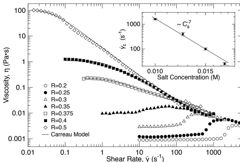
**Figure 3–1: Shear viscosity of CTAB/NaSal samples, vs. shear rate with  $R$  varying from 0.20 to 0.50. CTAB concentration was fixed at 0.05 M. Temperature was maintained at 25 °C. Lines represent fits to the Carreau model. Inset: Log-log plot of critical shear rate  $\dot{\gamma}_c$  as a function of salt concentration  $C_s$  for CTAB samples. The solid line denotes the best power-law fit for  $\dot{\gamma}_c$ .**
