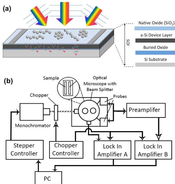
**Figure 5–1: (a) Schematic of the SOI device with nanoparticles. The ohmic aluminum contacts were deposited using thermal evaporation. Probes were used to apply a bias to the contacts. The nanoparticles were deposited through spin-coating. (b) Experimental current collector schematic.**
