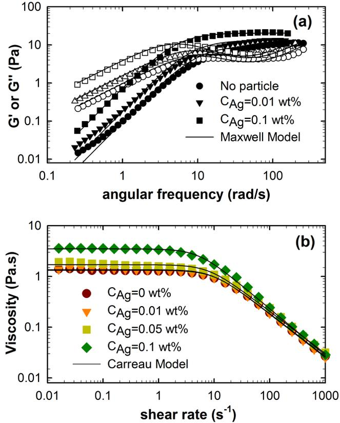
**Figure 2–4: a) Linear viscoelastic spectrum of 100 mM CTAB and 200 mM NaNO<sub>3</sub> as a function of Ag NPs weight fraction (Storage modulus,  $G'$ , closed symbols and loss modulus,  $G''$ , open symbols). Lines represent fits to the Maxwell model. b) Steady state viscosity of a wormlike micellar solution of 100 mM CTAB and 200 mM NaNO<sub>3</sub> as a function of Ag NPs weight fraction. Lines represent fits to the Carreau model.**
