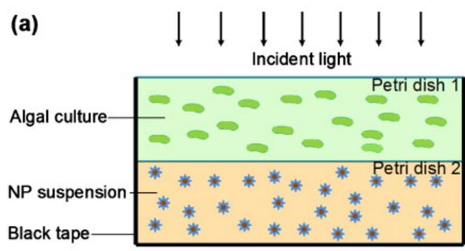
**Figure 5–6: Schematic of mini-photobioreactor using silver nanoparticles (Reprinted with permission from ref [37]. Copyright 2010 American Institute of Physics).**
