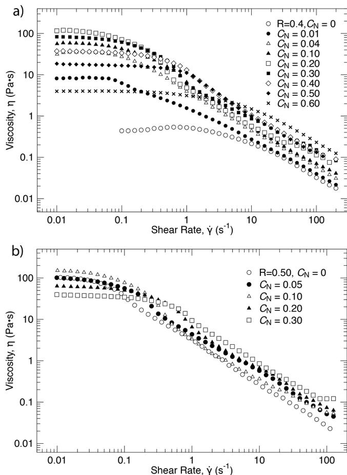
**Figure 3–5: Log-log plot of viscosity vs. shear rate for (a)  $C_D = 0.05$  M and  $R = 0.40$  with different concentrations of Ag nanoparticle addition. (b)  $C_D = 0.05$  M and  $R = 0.50$  with different concentrations of Ag nanoparticle addition.**
