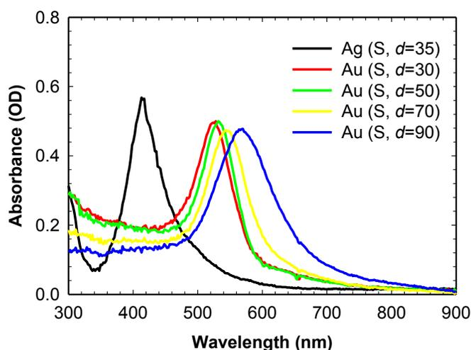
**Figure 2–5: Plasmonic response spectrum of spherical Au and Ag NPs of various diameter ( $d$ ) suspended in WLMs.**
