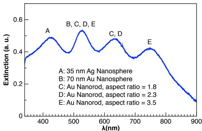
**Figure 2–8: A multicomponent plasmonic nanogel with a relatively uniform extinction spectrum over the visible range. Five different NPs (A-E) are suspended in the nanogel. Nanoparticles are distributed in the wormlike micellar solution of 100 mM CTAB/200 mM NaNO<sub>3</sub>.**
