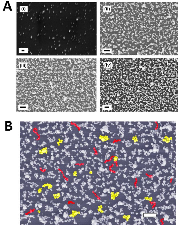
**Figure 5–4: (a) SEM images of (1) 0.1%, (2) 1%, (3) 5%, and (4) 10% w/v solutions on SOI wafer. (b) SEM of 1% w/v Ag solution on SOI with example strings (red) and clusters (yellow) colorized. All scale bars are 200 nm.**
