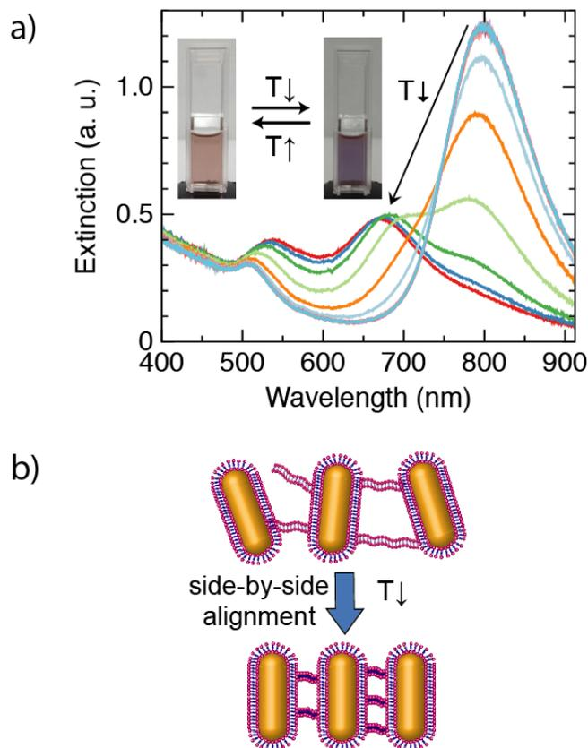
**Figure 4–2: Thermal tuning of plasmonic properties of colloidal Au nanorods. a) Au nanorod suspension switches between a disordered and an ordered state in response to temperature change. b) Hypothesized side-by-side alignment of Au nanorods due to the temperature change.**
