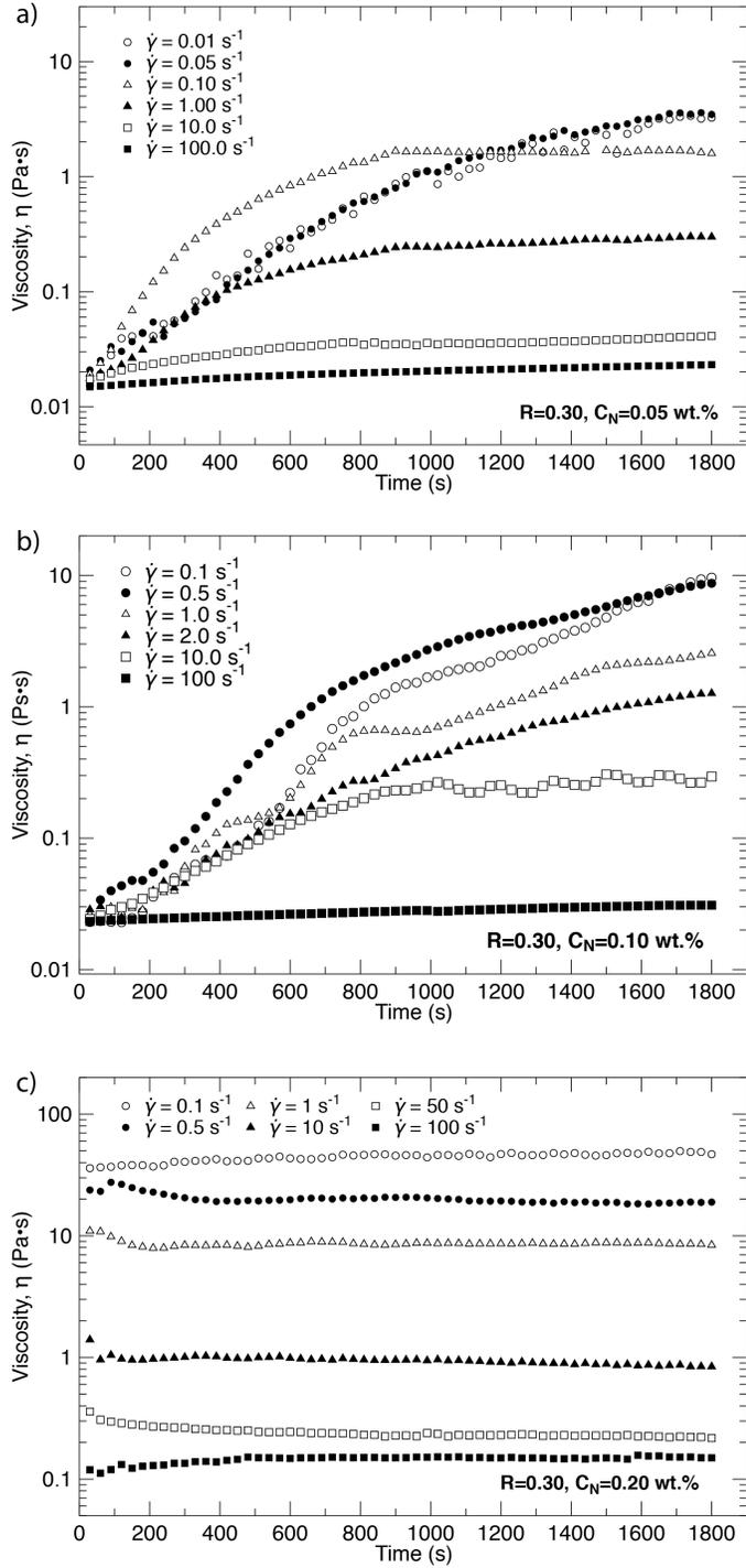
**Figure 3–2: Plot of viscosity vs. time for (a)  $R = 0.30$  and  $C_N = 0.05 \text{ wt.}\%$ , (b)  $R = 0.30$  and  $C_N = 0.10 \text{ wt.}\%$ , and (c)  $R = 0.30$  and  $C_N = 0.20 \text{ wt.}\%$  at different shear rates in Peak Hold experiments.**
