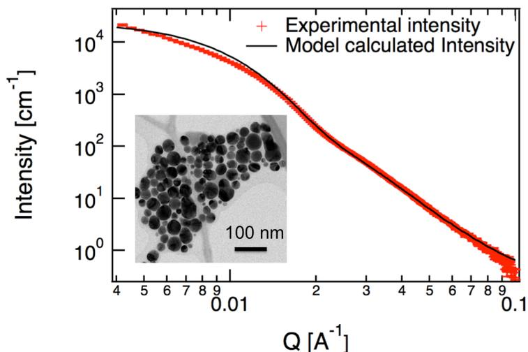
**Figure 2–2: Red symbol represents scattering intensity from PNG with 0.1 wt.% polydisperse Ag NPs (after subtract background). Solid line represents fitting using spherical model for particles with lognormal size distribution. Fitted particle diameter  $41 \pm 16$  nm. Inset: Transmission electron microscopy image of the polydisperse Ag NPs used in the experiment.**
