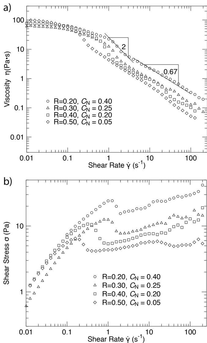
**Figure 3–8: Steady shear rheology of CTAB samples containing Ag nanoparticles with saturated network. CTAB concentration is 0.05 M. (a) Log-log plot of viscosity vs. shear rate. (b) Log-log plot of shear stress vs. shear rate.**
