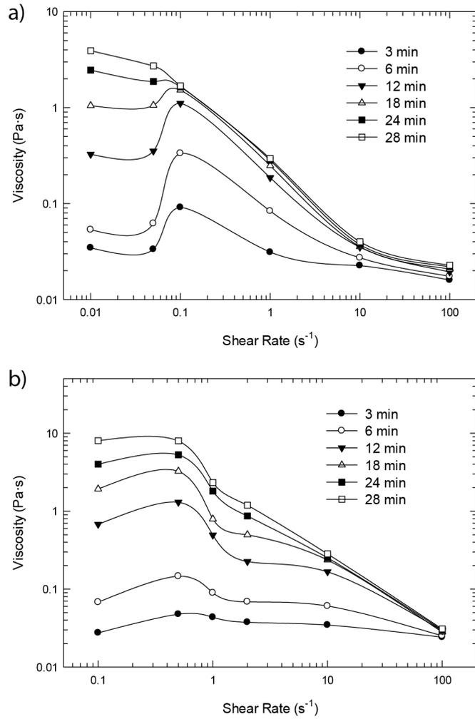
**Figure 3–3: Plot of viscosity vs. shear rate for (a)  $R = 0.30$  and  $C_N = 0.05 \text{ wt.}\%$  and (b)  $R = 0.30$  and  $C_N = 0.10 \text{ wt.}\%$  at different time in Peak Hold experiments. Lines are guide to eye.**
