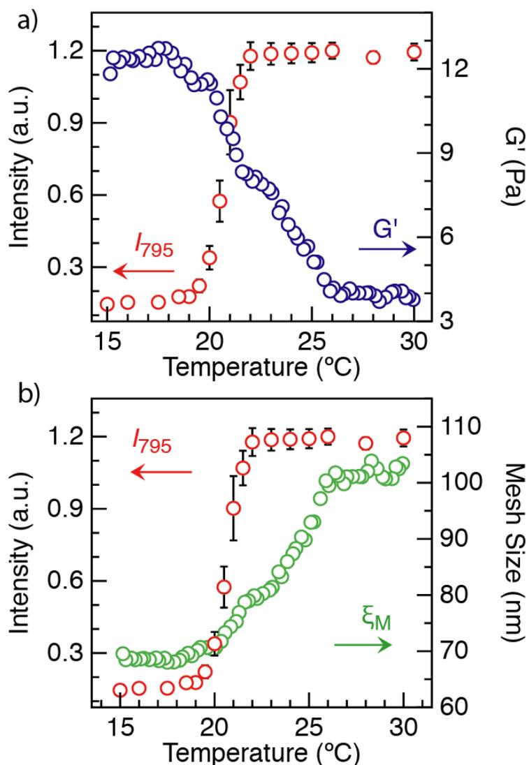
**Figure 4–7:** a) The relationship between extinction intensity at 795 nm and elastic modulus of a Au nanorods plasmonic micellar sample as a function of temperature. b) The relationship between extinction intensity at 795 nm and the calculated mesh size of entangled nanoparticle-mediated network as a function of temperature.
