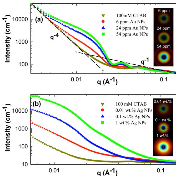
**Figure 2–3: a) SAXS data for plasmonic gels with 30 nm Au NPs. b) SAXS data for plasmonic gels with polydisperse Ag NPs.**
