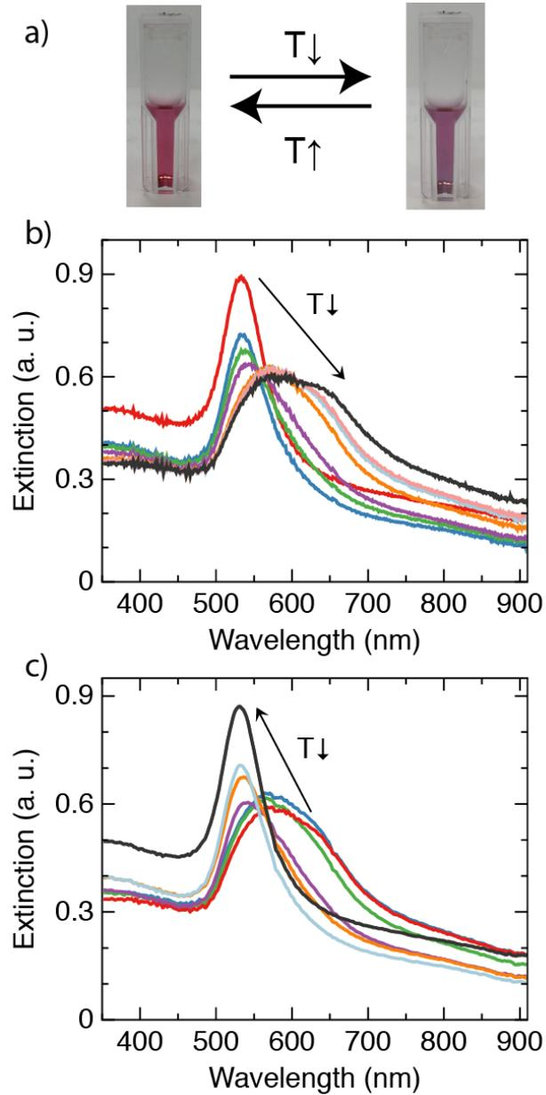
**Figure 4–1: Thermal tuning of plasmonic properties of colloidal Au nanospheres. a) Au nanosphere suspension switches between a disordered and an ordered state in response to temperature change. b) The extinction spectra of a typical Au nanosphere suspension when cooled from 30 °C to 15 °C, and c) the extinction spectra of the same sample when heated from 15 °C back to 30 °C.**
