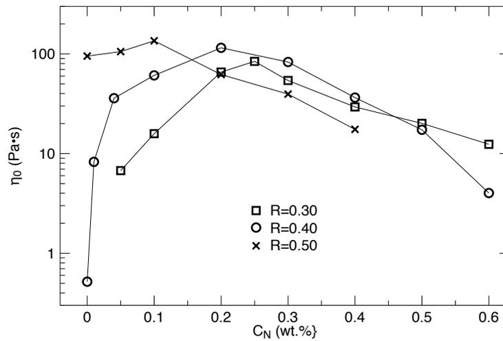
**Figure 3–6: Plot of zero shear viscosity vs. shear rate for  $C_D = 0.05$  M and  $R = 0.30$ ,  $R = 0.40$  &  $R = 0.50$  with different concentrations of Ag nanoparticle addition. Lines are only guide to eye.**
