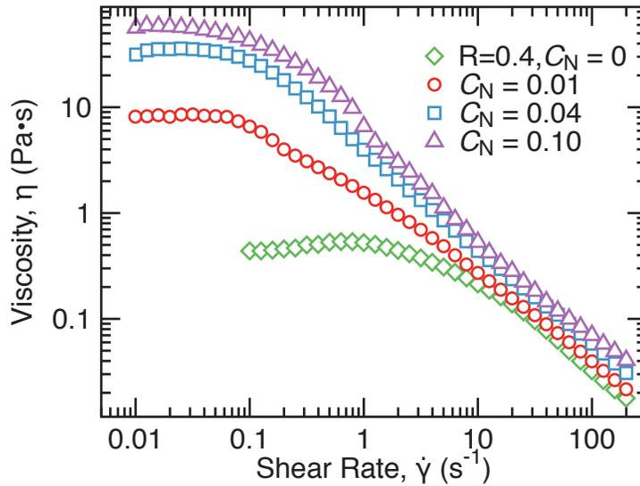
**Figure 5–11: Viscosity of plasmonic nanogel with different Ag NP concentration vs. shear rate. CTAB concentration is 50 mM and NaSal concentration is 20 mM.**
