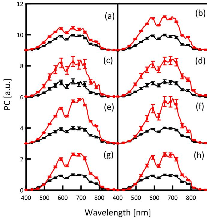
**Figure 5–2: Photocurrent response of (a) 0.01%, (b) 0.05%, (c) 0.1%, (d) 0.2%, (e) 0.5%, (f) 1%, (g) 5%, and (h) 10% wt./vol. Ag nano ink coatings. The bare SOI wafers have been normalized for comparison. Error bars show the standard error for the measurements Photocurrent measurements are offset by 3 for display.**
