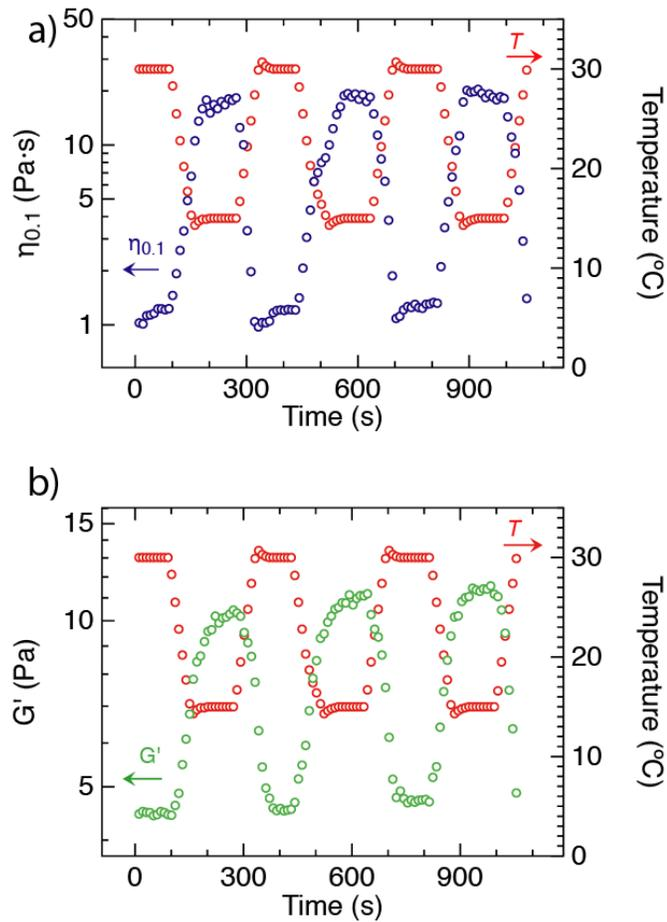
**Figure 4-5: The thermoreversible rheological response of a plasmonic micellar solution. The temperature is controlled via a preset procedure and the resulting viscosity at a shear rate of  $0.1 \text{ s}^{-1}$ ,  $\eta_{0.1}$  and the apparent elastic modulus  $G'$  are recorded as a function of time.**
