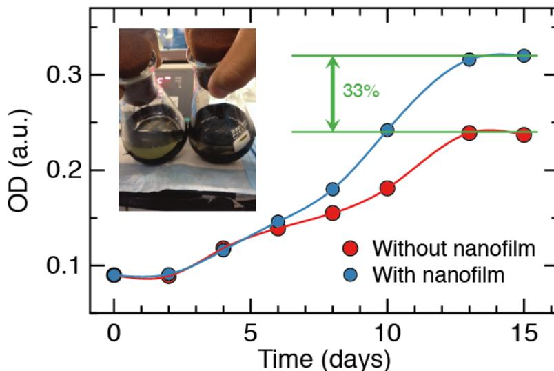
**Figure 5–9: Experimentally observed algae concentration as a function of time. The inset shows photograph of the cultured algae species *C. Reinhardtii* in photobioreactor with (left) and without (right) plasmonic nanofilm after 15 days.**
