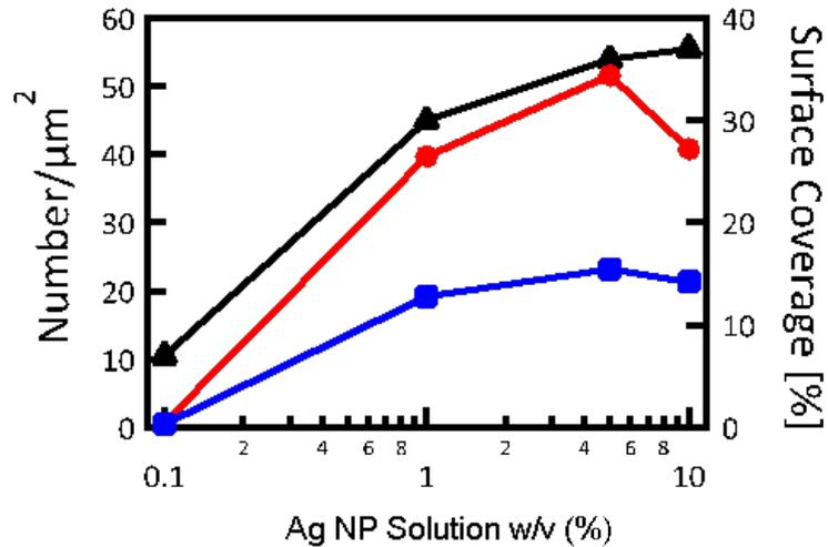
**Figure 5–5: Silver solution w/v vs. the 40 nm particle surface coverage (black line) and number of particle formations. The number of clusters (red line) and the number of strings (blue line) are shown per  $\mu\text{m}^2$ .**
