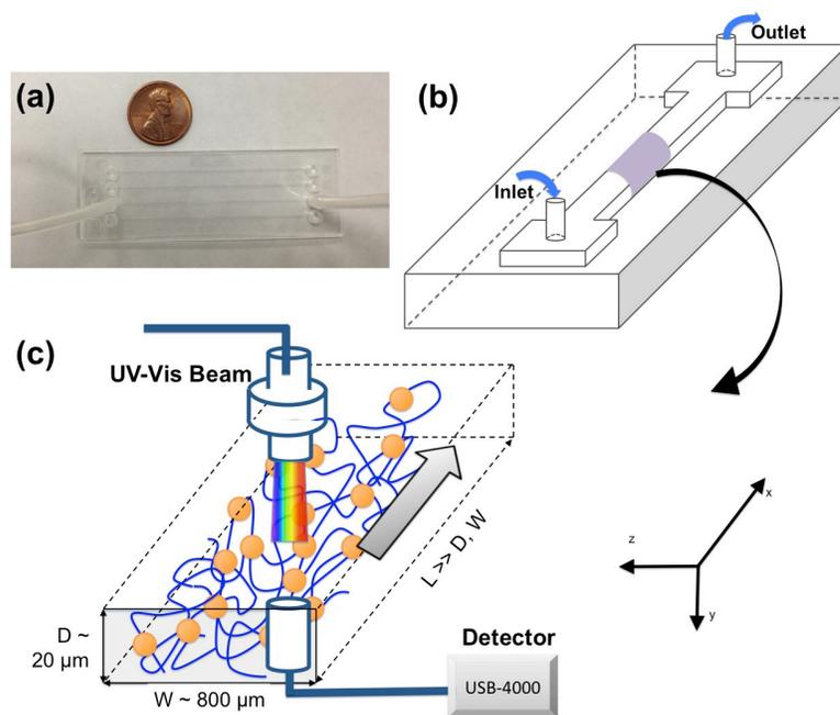
**Figure 5–10: (a) Microfluidic channel fabricated by PMMA. (b) Schematic representation of the microfluidic channel. (c) Magnified view of the region within the channel where the UV-Vis spectrometer with an integrated optical fiber is located to record the optical signal.**
