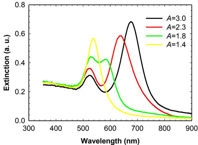
**Figure 2–6: Plasmonic response spectrum of rod-like Au NPs ( $d_{\text{rod}} = 25$  nm) with various aspect ratios ( $A$ ) suspended in WLMs.**
