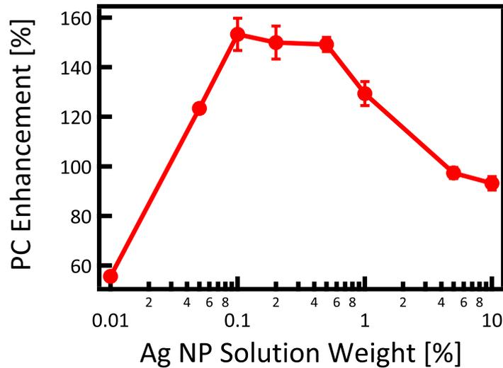
**Figure 5–3: Silver ink solution wt./vol. vs. overall photocurrent enhancement. Error bars show the standard error for the measurements.**
