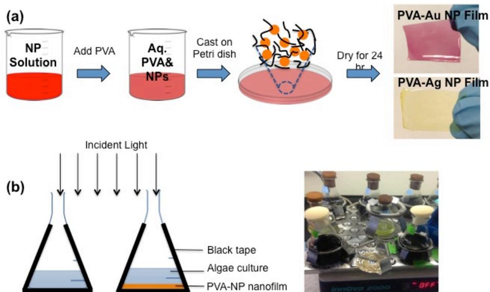
**Figure 5–7: (a) Schematic representation of PVA-NP nanofilms manufacturing process. (b) Schematic of nanofilms wrapped photobioreactor and a photo of experimental setup.**
