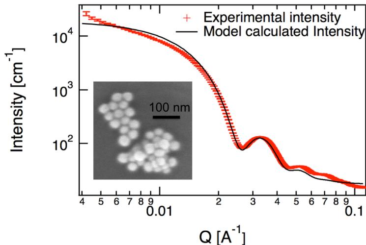
**Figure 2–1: Red symbol represents scattering intensity from PNG with 54 ppm monodisperse Au NPs (after subtract background). Solid line represents fitting using spherical model for particles with lognormal size distribution. Fitted particle diameter  $32 \pm 3.2$  nm. Inset: Scanning electron microscopy image of the monodisperse Au NPs used in the experiment.**
