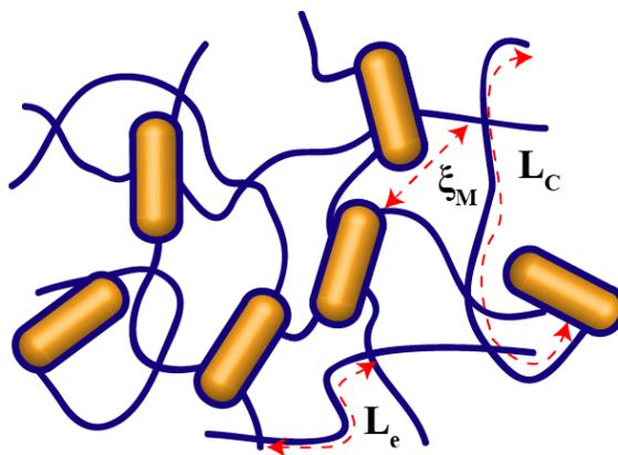
**Figure 4–6: Illustration of a nanoparticle mediated entangled micellar network and associated length scales.**
