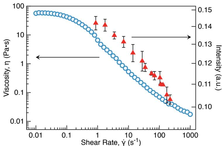
**Figure 5–13: Apparent viscosity and absorption peak intensity at  $\sim 410$  nm as a function of applied shear rate. Open circles denote viscosity data and solid triangles with error bars denote plasmon resonance peak intensity.**
