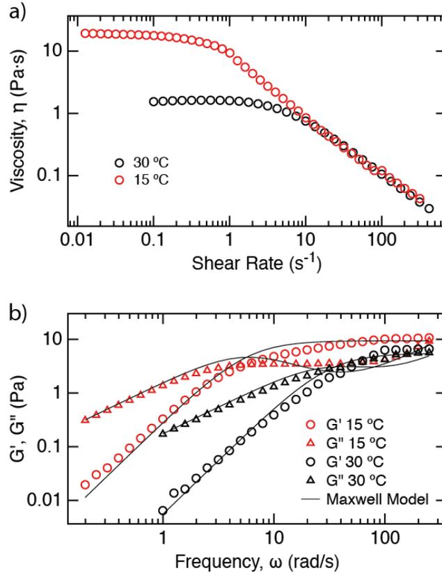
**Figure 4-4: a) Steady state viscosity of an Au nanorod suspension in wormlike micellar solution at different temperatures. b) Linear viscoelastic spectrum of an Au nanorod suspension in wormlike micellar solution at different temperatures (Storage modulus,  $G'$ , cycle and loss modulus,  $G''$ , triangle). Lines represent fits to the Maxwell model.**
