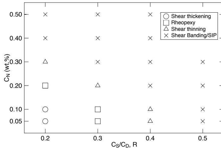
**Figure 3–9: Diagram of rheological behaviors of the CTAB/NaSal/Ag NP solutions. Shear thickening, rheopexy, and shear thinning are shown in circles, squares, and triangles respectively. Cross symbols denote regions in which shear banding or shear induced phase separation are observed.**
