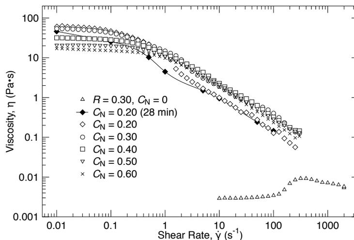
**Figure 3–4: Log-log plot of viscosity vs. shear rate for  $C_D = 0.05$  M and  $R = 0.40$  with different concentrations of Ag NP addition. Filled diamond symbols denote the viscosity measured at 30 min in Peak Hold experiment. Lines are guide to eye.**
