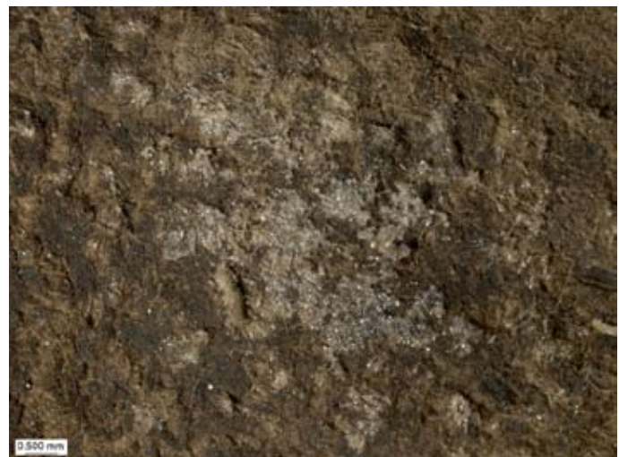
Figure 3. Leather substrate bearing a thin, crystalline coating (Photo: Mel Wachowiak and Maria Fusco, Museum Conservation Institute, Smithsonian Institution).
