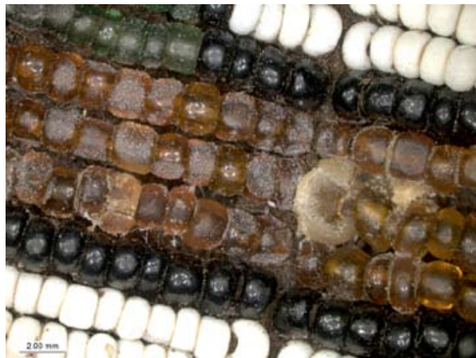
Figure 6. Unstable glass bearing an engulfing, opaque coating. Qualitative glass compositional analyses and identification of degradation products were undertaken with \mu -XRF (Photo: Mel Wachowiak and Maria Fusco, Museum Conservation Institute, Smithsonian Institution).
