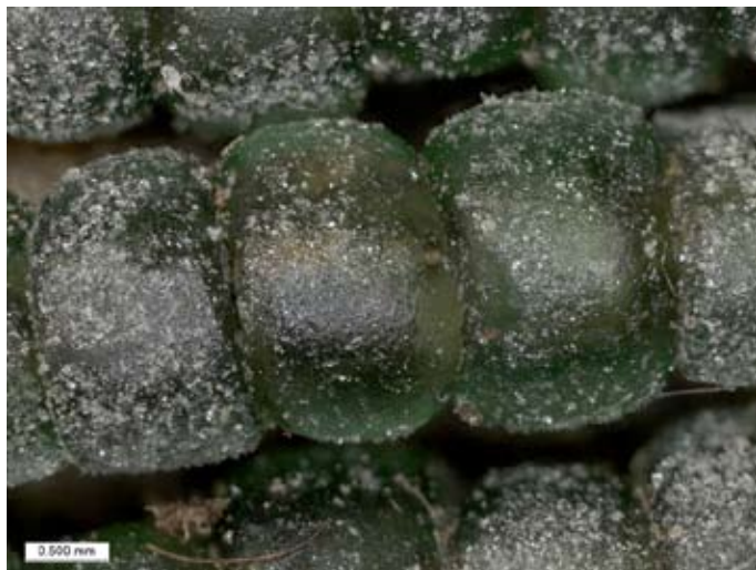
Figure 4. Stable glass bearing a thin “sugary” coating. Qualitative glass compositional analyses were undertaken with \mu -XRF (Photo: Mel Wachowiak and Maria Fusco, Museum Conservation Institute, Smithsonian Institution).
