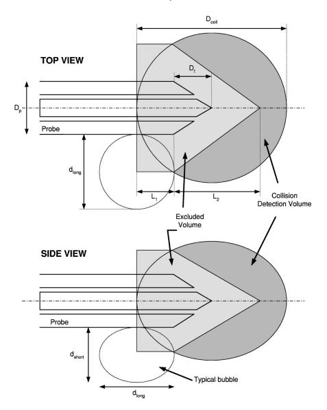
FIG. 8. Sketch of the geometry of the probe excluded volume and bubble collision detection volume.
