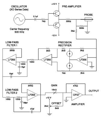
FIG. 2. Electronics schematic diagram.
