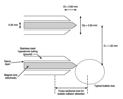
FIG. 1. Sketch of the dual impedance probe.
