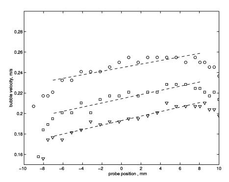
FIG. 14. Bubble velocity profiles for three typical hold ups. ( $\bigcirc$ ),  $\alpha$ =0.02; ( $\square$ ),  $\alpha$ =0.05; and ( $\nabla$ ),  $\alpha$ =0.10, for a channel inclination of  $\theta$ =5°. The lines show the linear best fits.
