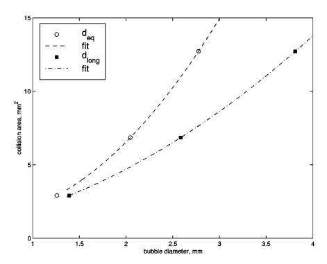
FIG. 9. Measured collision area as a function of the bubble equivalent diameter  $d_{\rm eq}$  and bubble's long axis  $d_{\rm long}$ . Lines show the fit to the measurements
