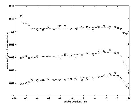
FIG. 10. Gas fraction profiles for three typical hold ups. ( $\bigcirc$ ),  $\alpha$ =0.02; ( $\square$ ),  $\alpha$ =0.05; and ( $\nabla$ ),  $\alpha$ =0.10, for a channel inclination of  $\theta$ =5°. The lines show best linear fits of the data excluding the near-wall regions.
