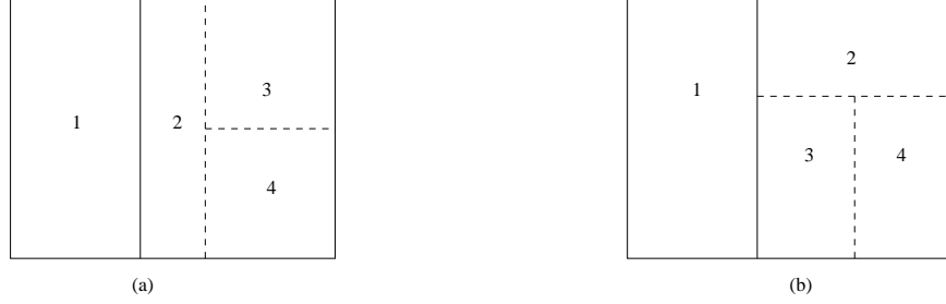
Figure 9: Decomposition in (b) can be achieved by rotating the dotted lines of decomposition in (a).
