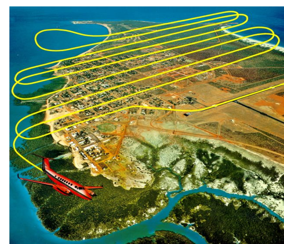
Figure 2. Flight Plan Illustration. Created by BAKOSURTANAL (2006). (Personal Communication).
