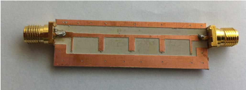
Figure 3.21: Fabricated Filter
