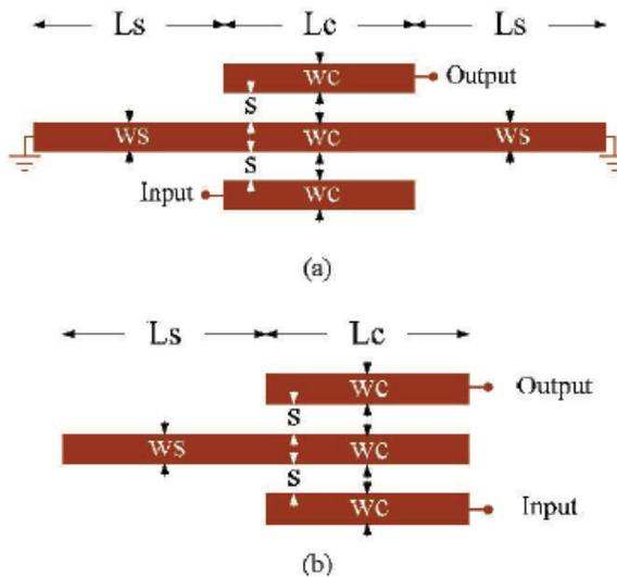
Figure 2.12: Multiline coupled line filter sample
