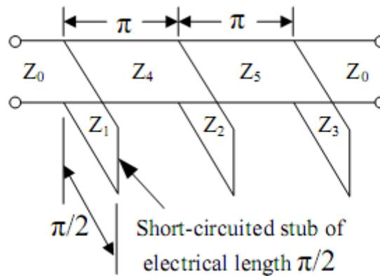
Figure 2.13: Quarter wavelength shorted stub separated by half wavelength lines
