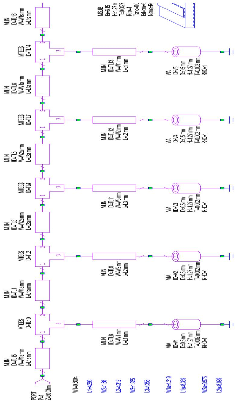
Figure 3.4: Initial AWR optimized circuit schematic
