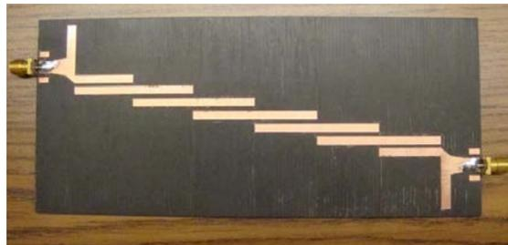
Figure 2.10: Filter sample with tapped input section (removed coupled input section)
