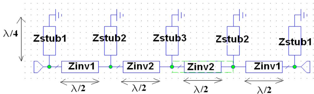
Figure 3.3: The design prototype of the filter
