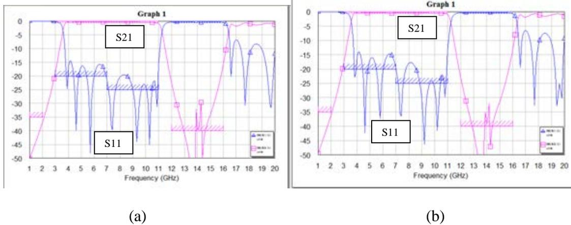
Figure 3.24: AWR Simulation Results due to tolerance analysis (series lines' widths)
