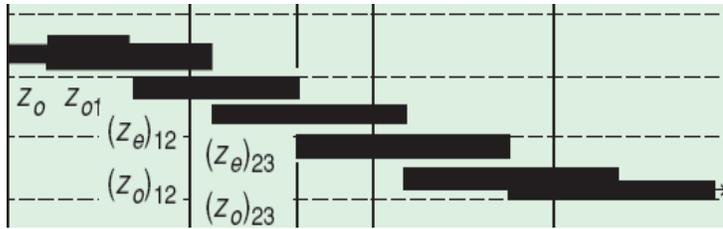
Figure 2.11: Coupled Lines with impedance transforming section
