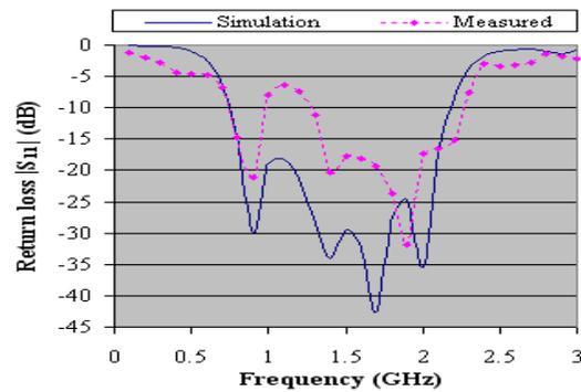
Figure 2.6: Filter using short circuited stubs: (a) Prototype, (b) Filter Performance
