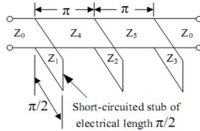
Figure 3.2: The structure of the shorted stub BPF
