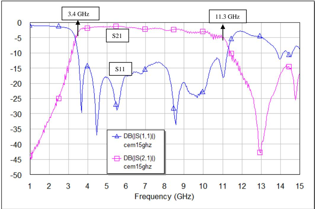
Figure 3.26: The final S-parameter measurements of the filter
